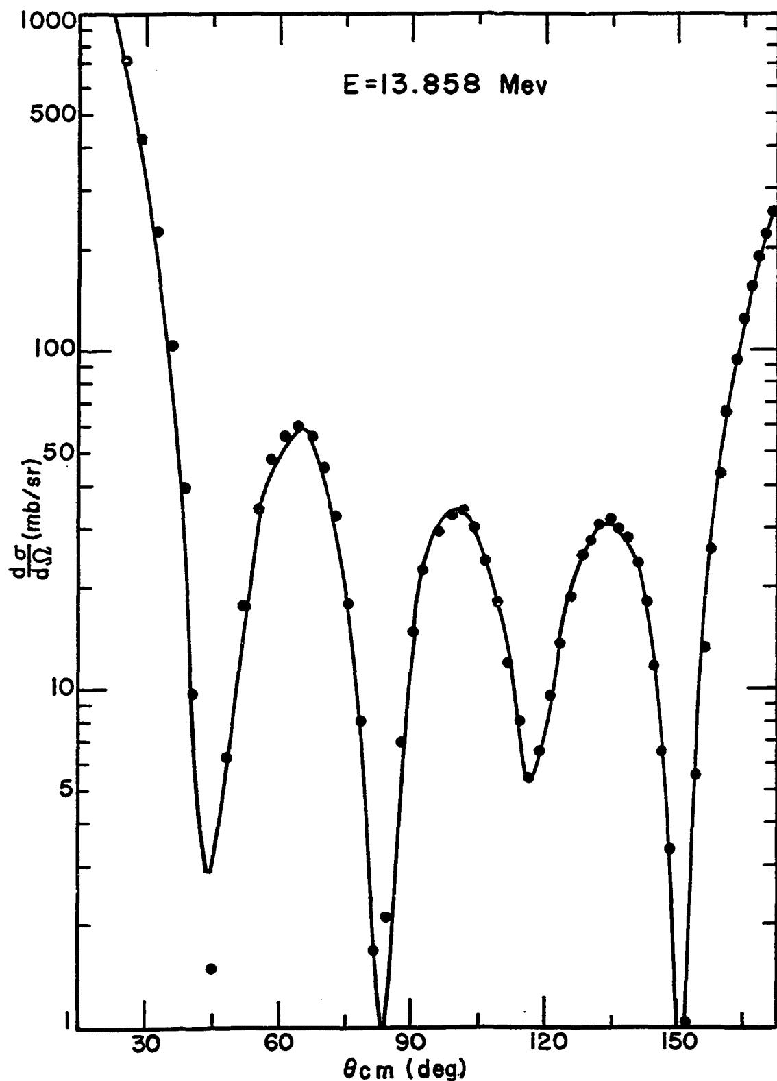
Figure 11. Fit to angular distribution at an alpha-particle energy of 13.858 Mev (● Experimental, — Calculated fit)
