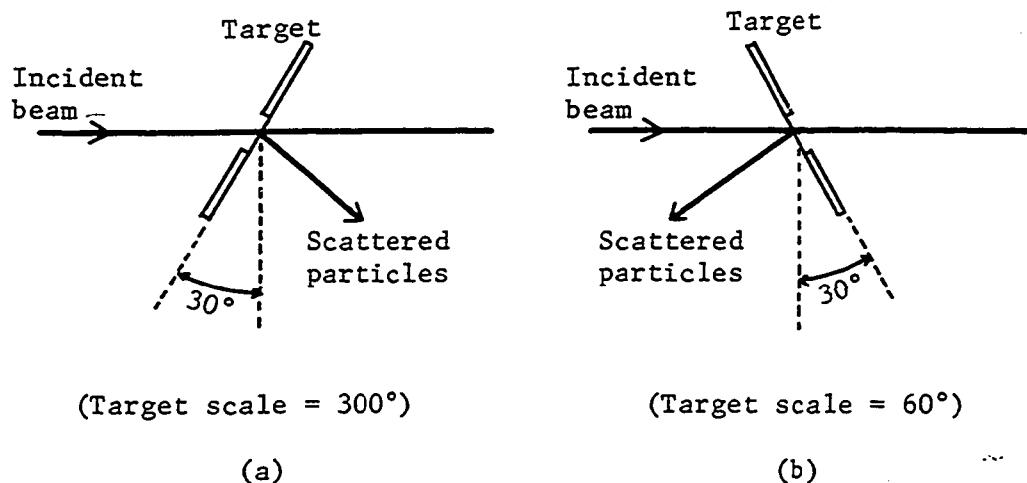
Figure 2. Target positions in taking excitation functions
