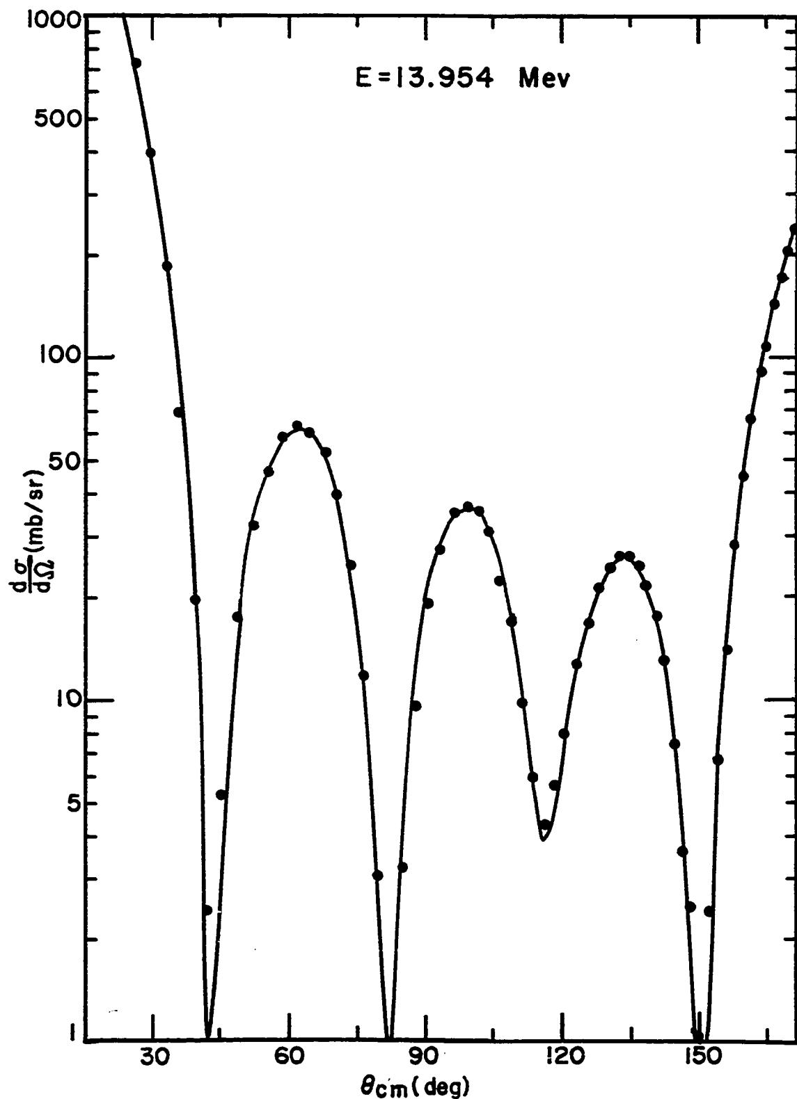
Figure 12. Fit to angular distribution at an alpha-particle energy of 13.954 Mev (● Experimental, — Calculated fit)
