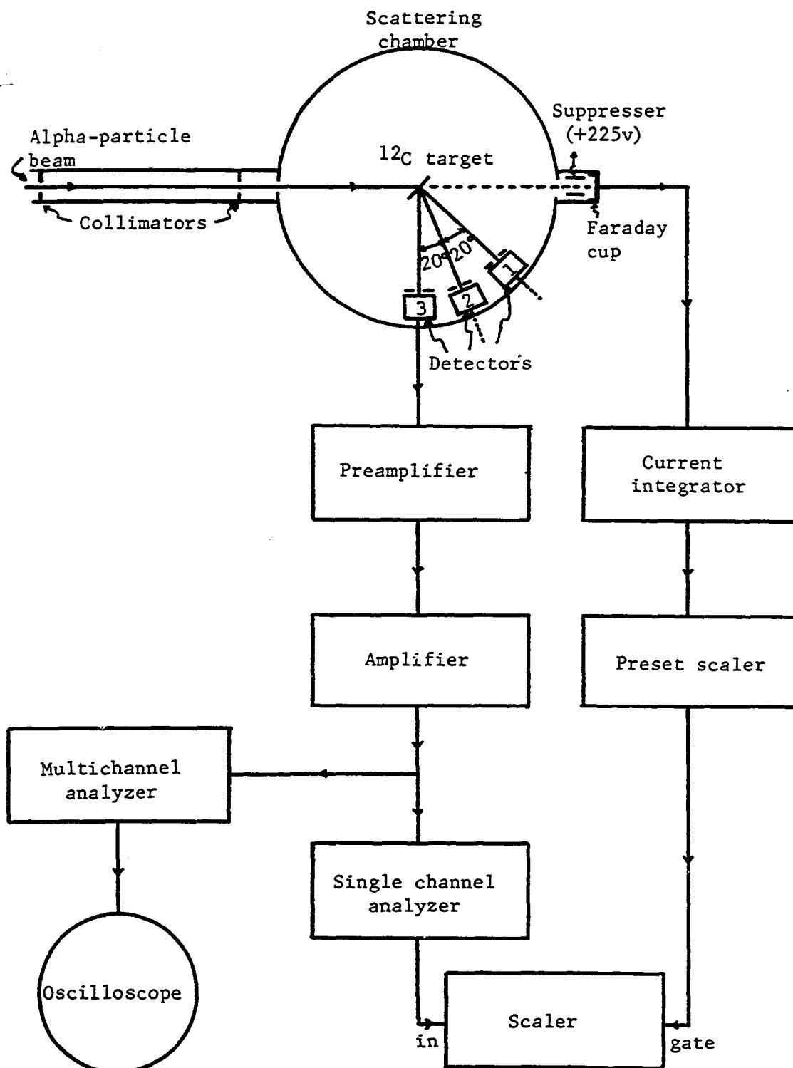
Figure 1. Electronics layout for data measurements
