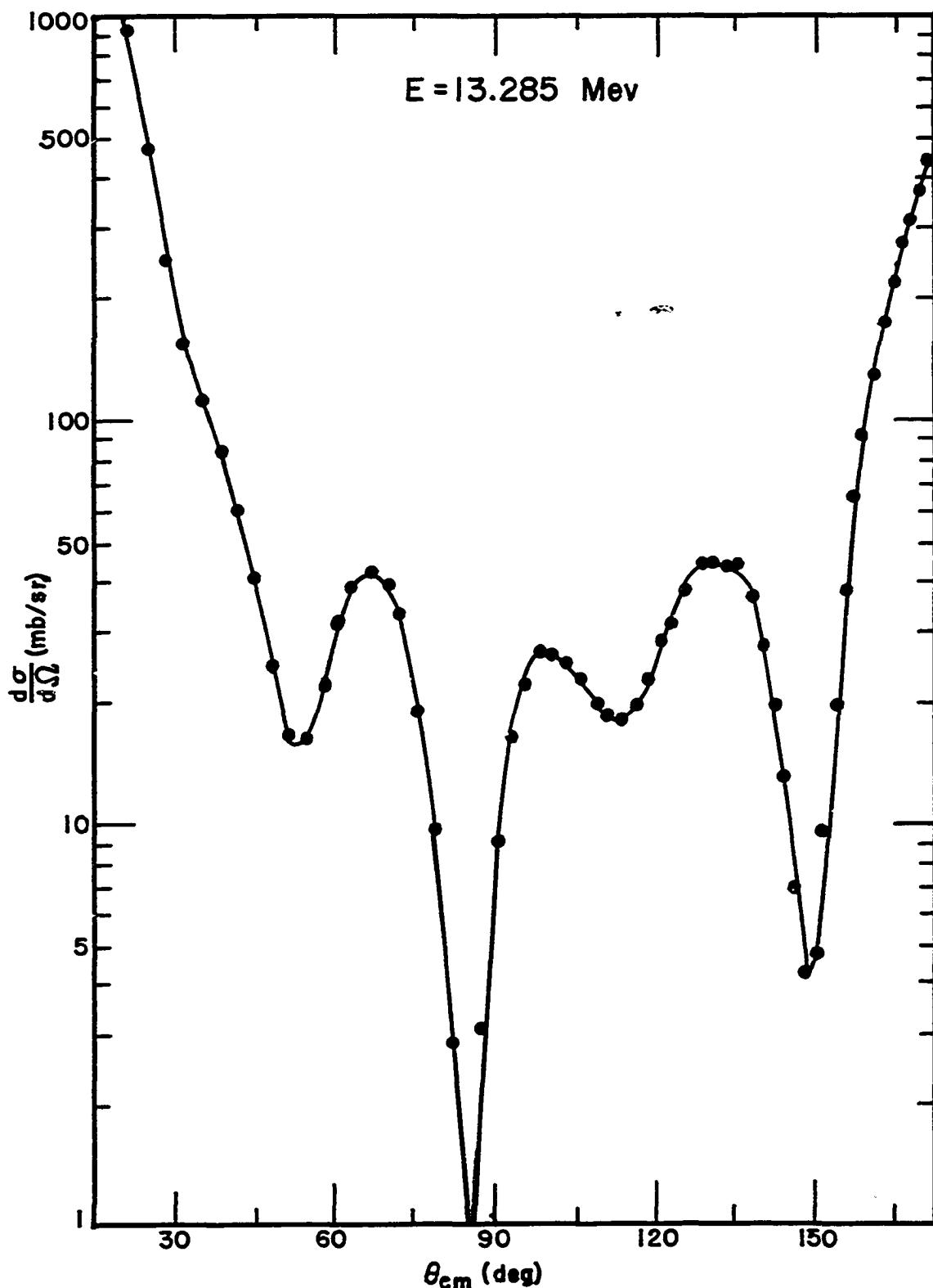
Figure 7. Fit to angular distribution at an alpha-particle energy of 13.285 Mev (● Experimental, — Calculated fit)
