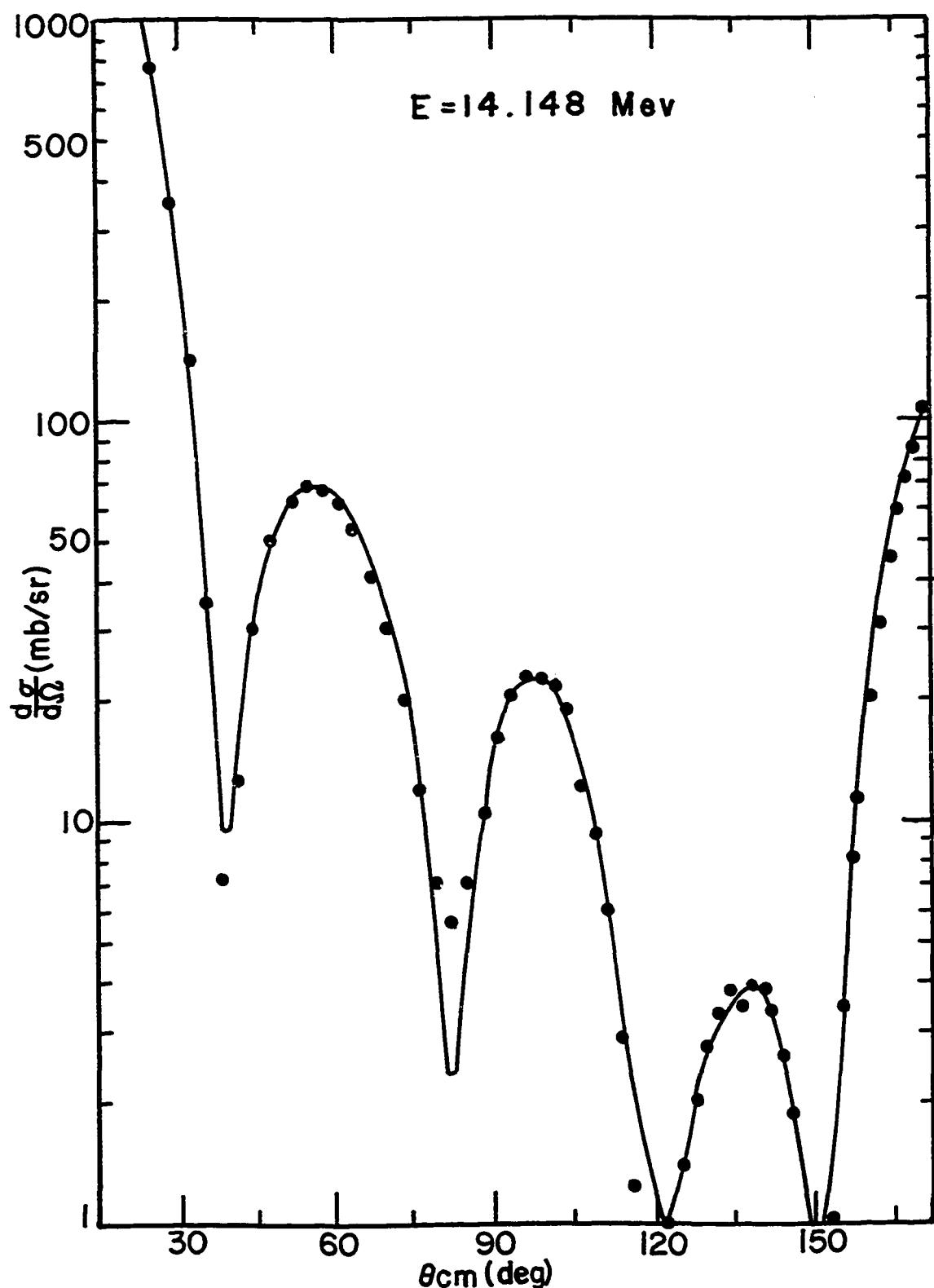
Figure 15. Fit to angular distribution at an alpha-particle energy of 14.148 Mev (● Experimental, — Calculated fit)
