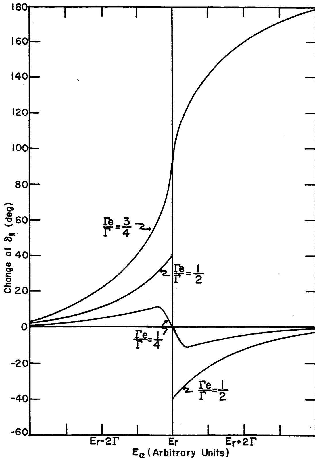
Figure 4. Variation in phase angles near the resonant energy
