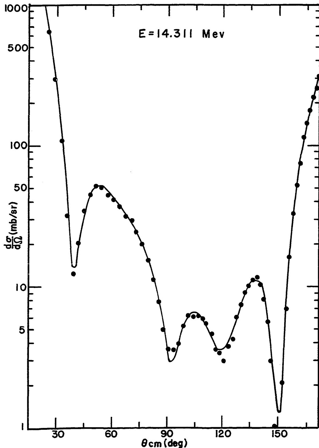
Figure 16. Fit to angular distribution at an alpha-particle energy of 14.311 Mev (● Experimental, — Calculated fit)
