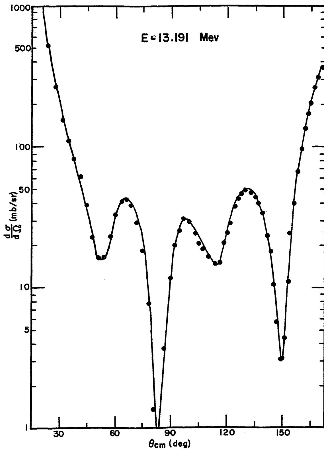
Figure 6. Fit to angular distribution at an alpha-particle energy of 13.191 Mev (● Experimental, — Calculated fit)
