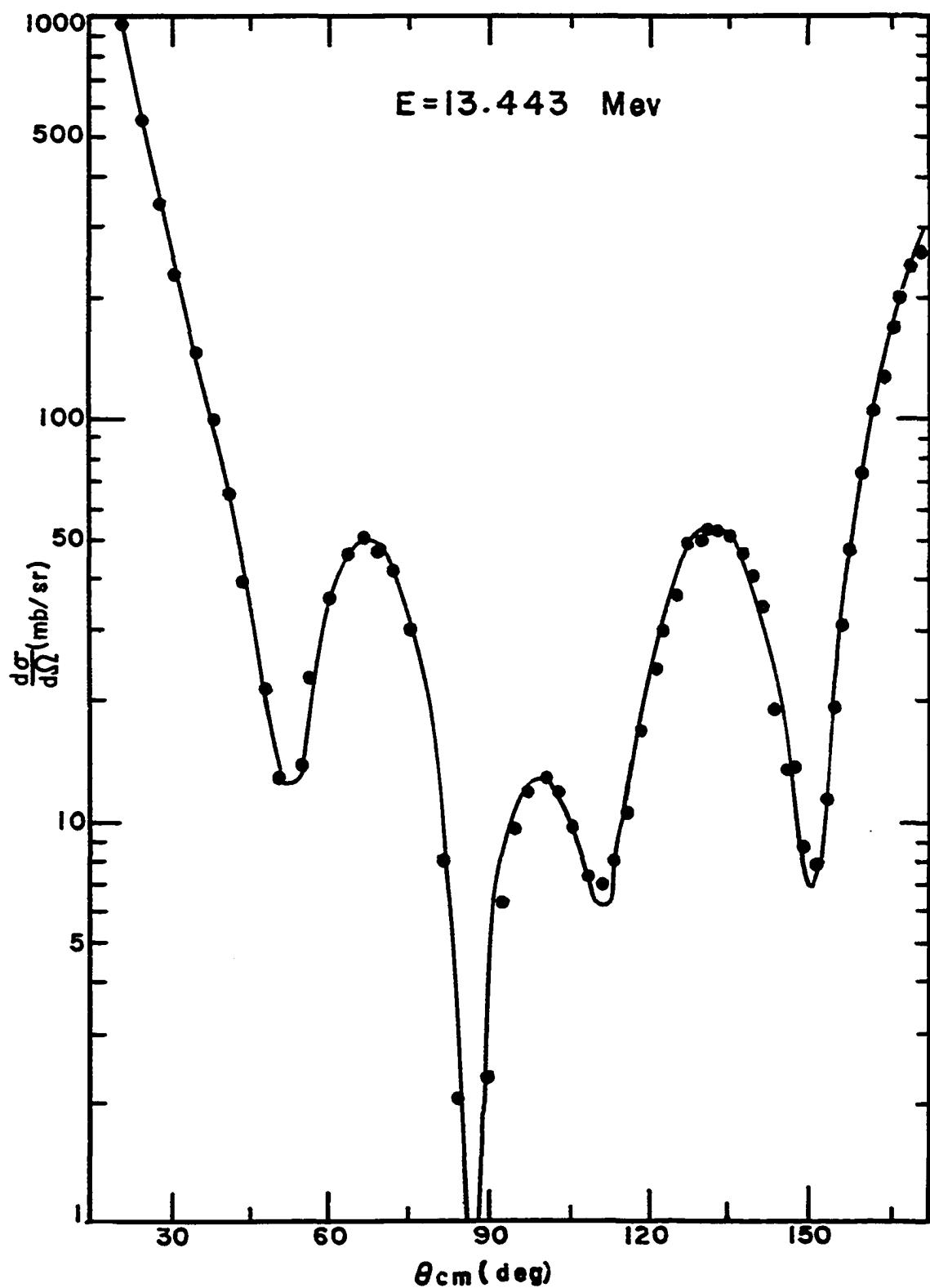
Figure 8. Fit to angular distribution at an alpha-particle energy of 13.443 Mev (● Experimental, — Calculated fit)
