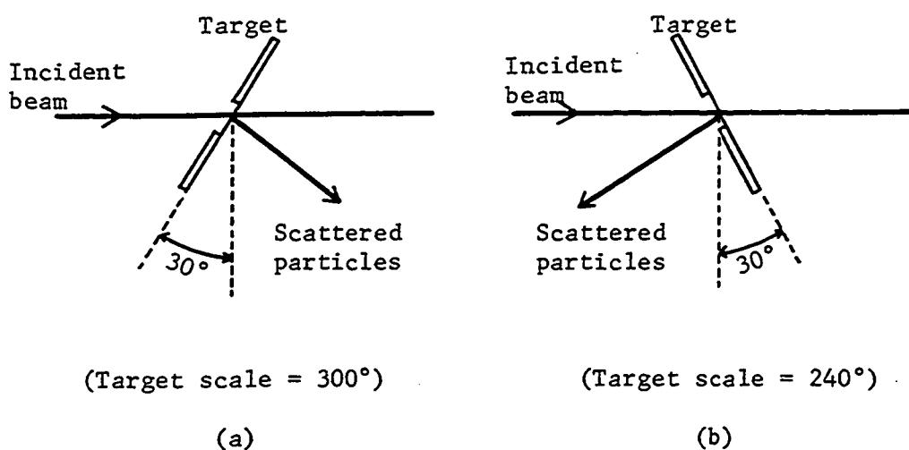
Figure 3. Target positions in taking angular distributions
