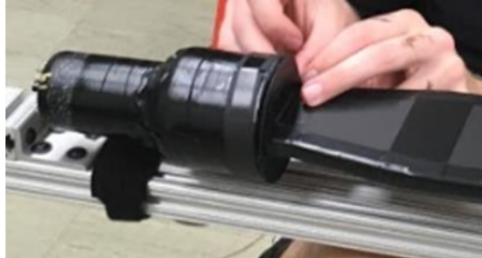
Figure 8. The finished product of the process that makes the scintillators "light tight". After having been painted in reflective paint, it is then wrapped in black vinyl as seen in the picture.
