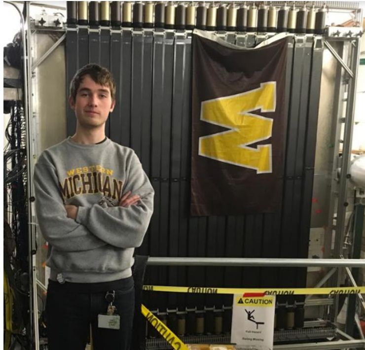
Figure 4 The Proton Veto Wall. It is the black vertical bars that the flag covers, in the background. Justin Swaim is pictured in the foreground of the photo. The detector itself is about 3 meters in height, and is situated in front of LANA (metal shielded surface behind the black scintillator bars).
