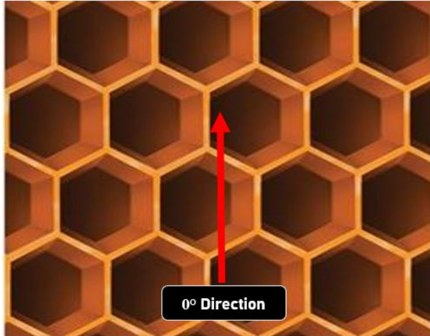
Figure 164 - 0° direction of honeycomb core
