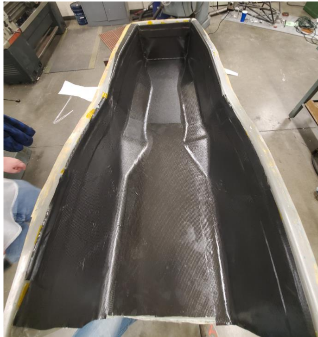
Figure 159 - B20 molds with first laminate finished
