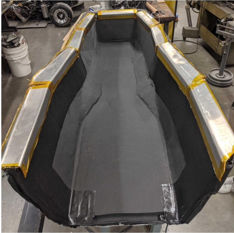
Figure 173 – BR20 Dams attached to molds
