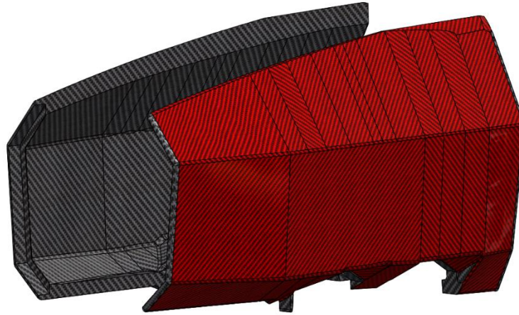
Figure 51 - FBHS Rules Regulated Region Moment of Inertia Calculation CAD
