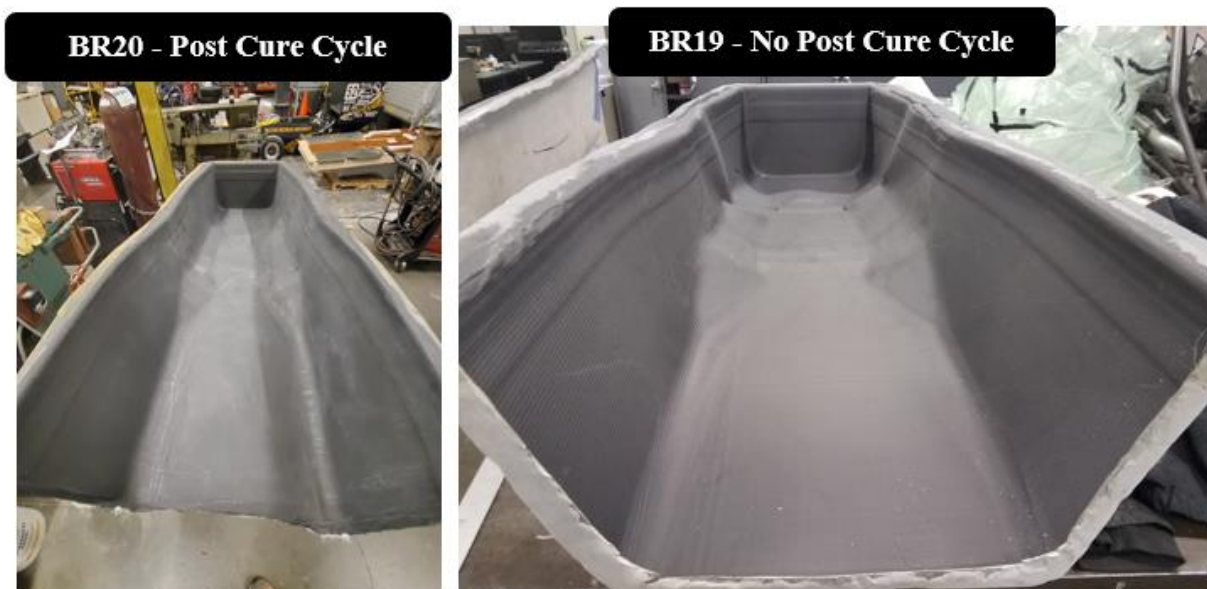
Figure 148 - Comparison of BR19 warped layup vs successful layup
