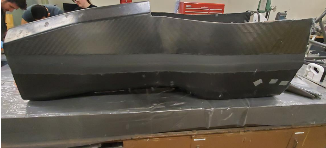
Figure 187 - BR20 with cured lap joint
