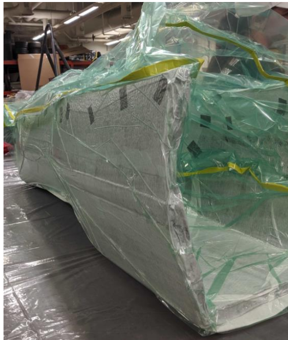
Figure 186 - Full BR20 monocoque bagged after lap joint
