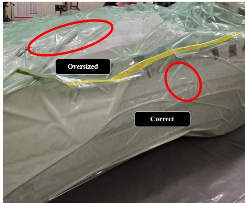
Figure 156 - Correct vs incorrect sized cleats
