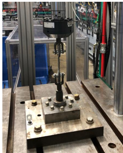
Figure 138 - Lap joint test setup
