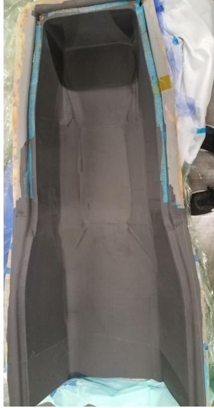
Figure 174 - Successful cure of B19 lower mold
