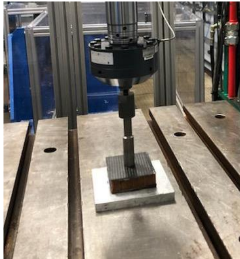
Figure 128 - Perimeter shear test setup
