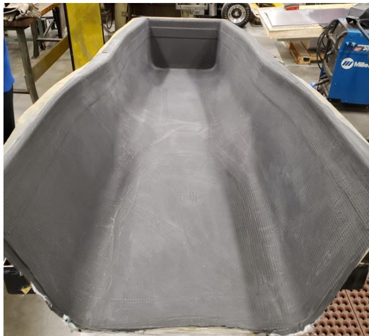
Figure 163 - First side of BR20 laminate cured
