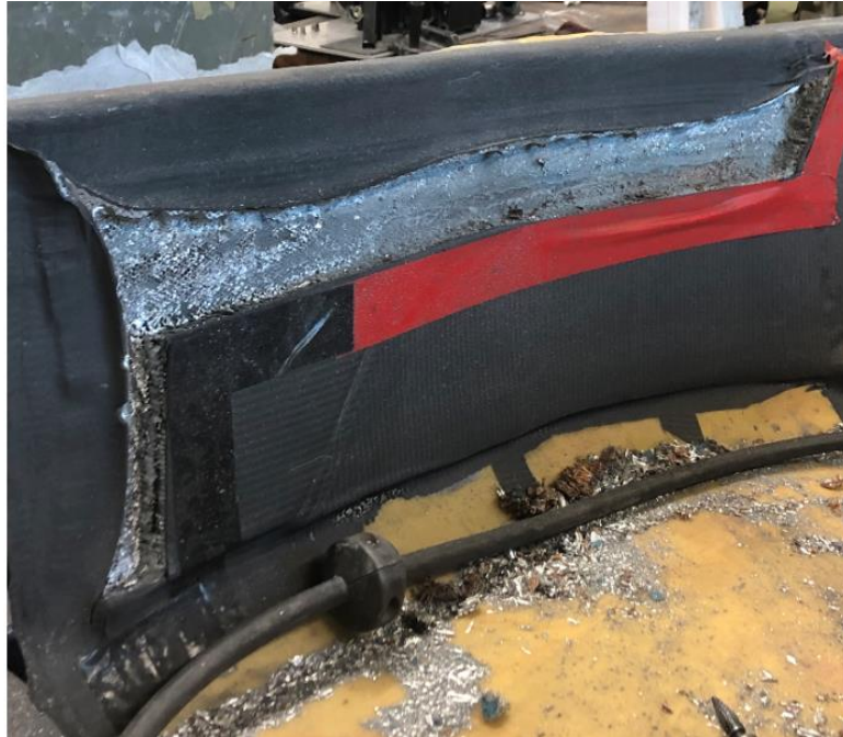
Figure 178 - Removed core of BR20 lower mold repair
