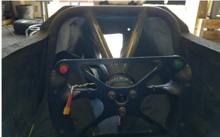
Figure 9 - Excessive front roll hoop height
