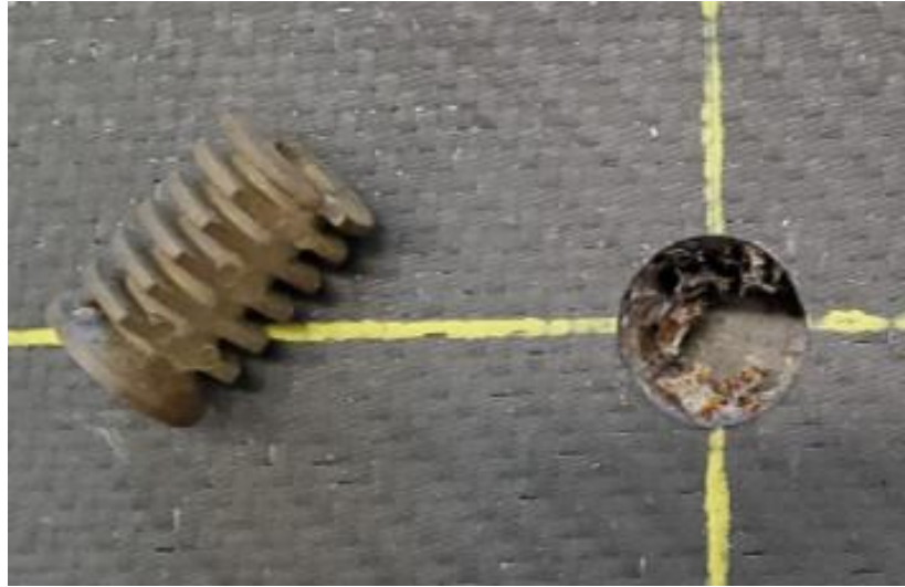
Figure 189 - Torlon insert and through hole
