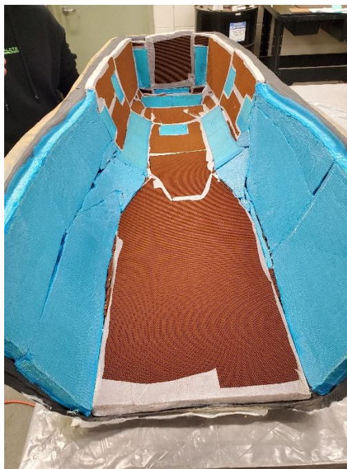
Figure 168 - BR20 with all aluminum and balsa core materials bonded in place
