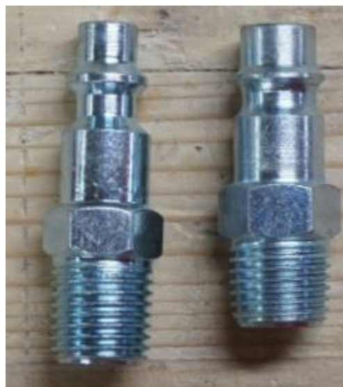
Figure 160 - Our quick disconnect fitting vs Pratt & Whitney's
