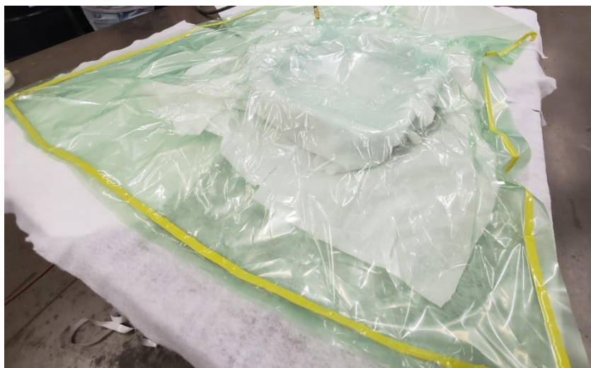
Figure 154 - Vacuum bag for monocoque
