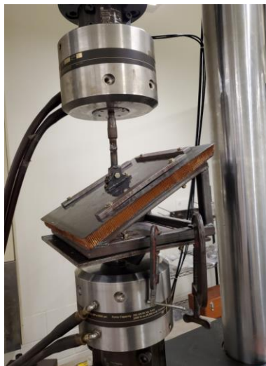
Figure 136 - Harness mount test setup
