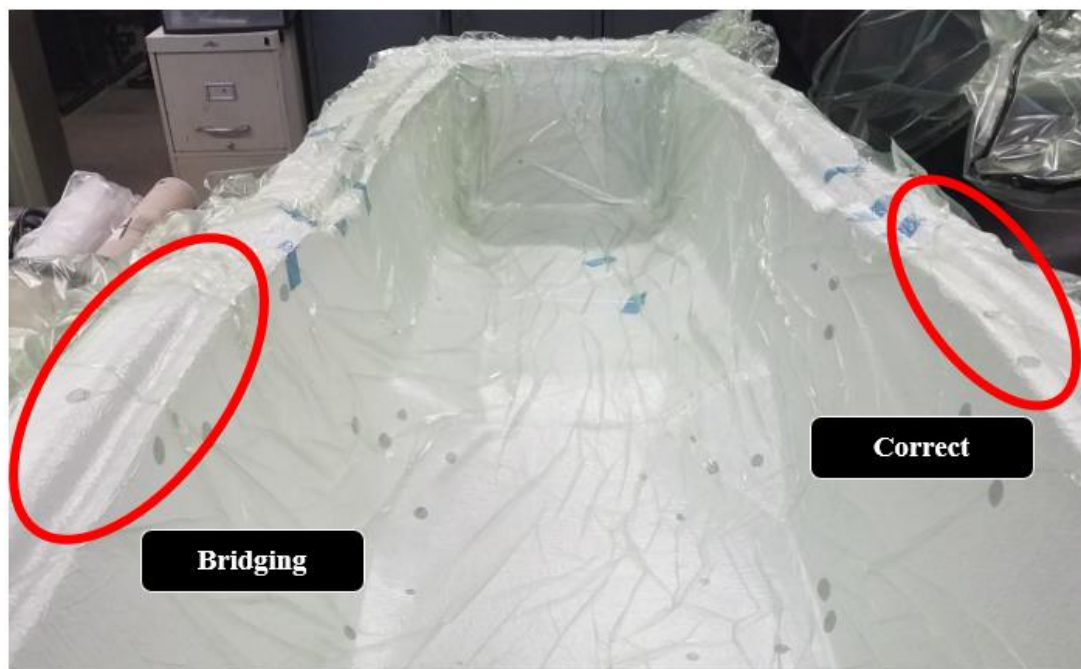
Figure 155 - Correct bagging vs bridged bagging
