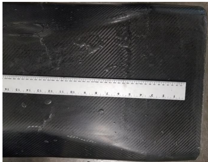
Figure 11 - BR19 monocoque bottom view after demolding
