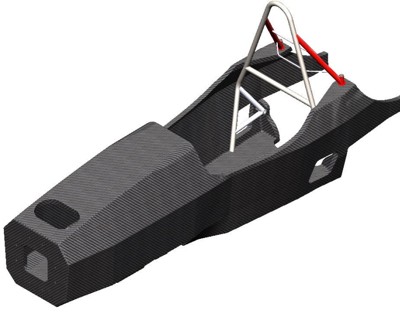
Figure 73 - Main roll hoop bracing highlighted
