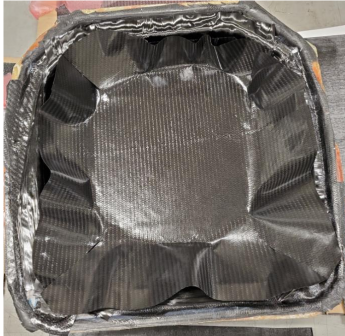
Figure 153 - Extreme bridging of BR20 front bulkhead
