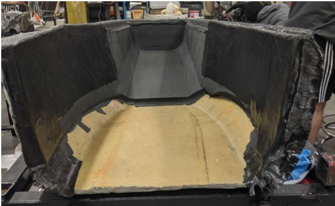
Figure 180 - BR20 uncured repair
