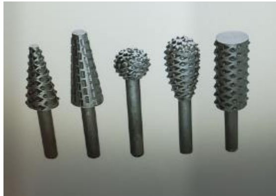
Figure 177 - Grinding bits to remove core
