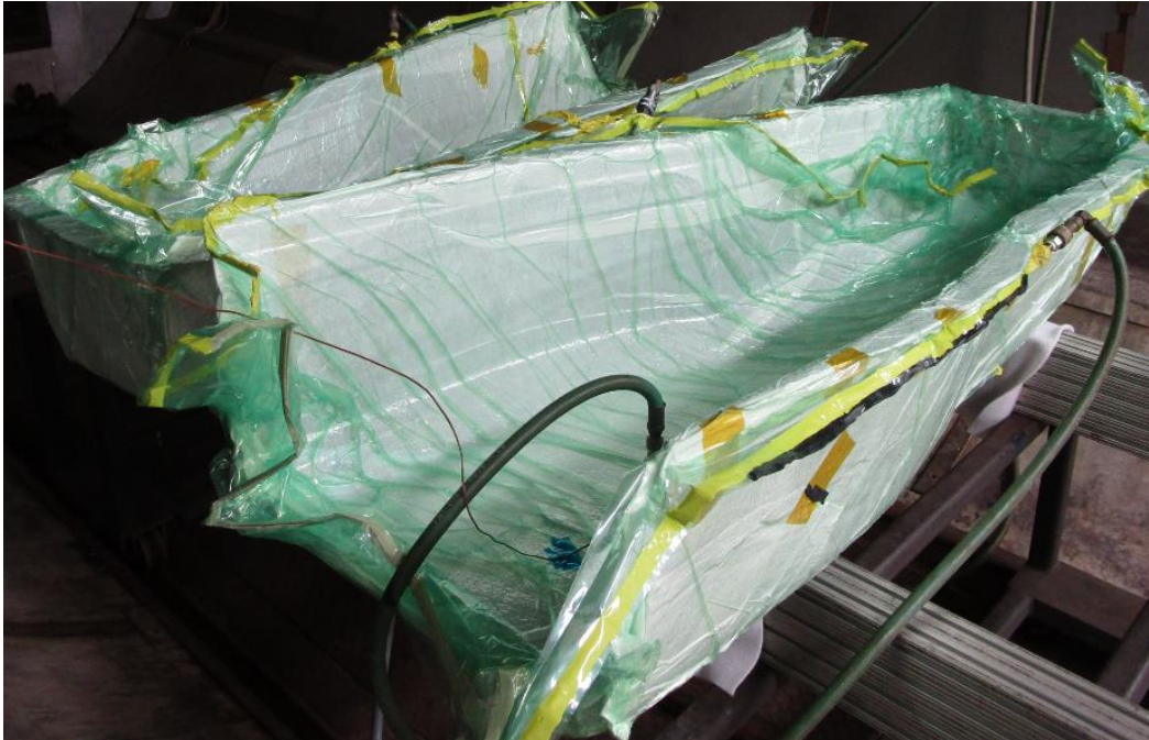
Figure 162 - Properly vacuum bagged mold for this stage
