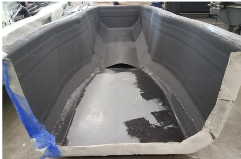
Figure 12 - Warped first iteration monocoque laminate
