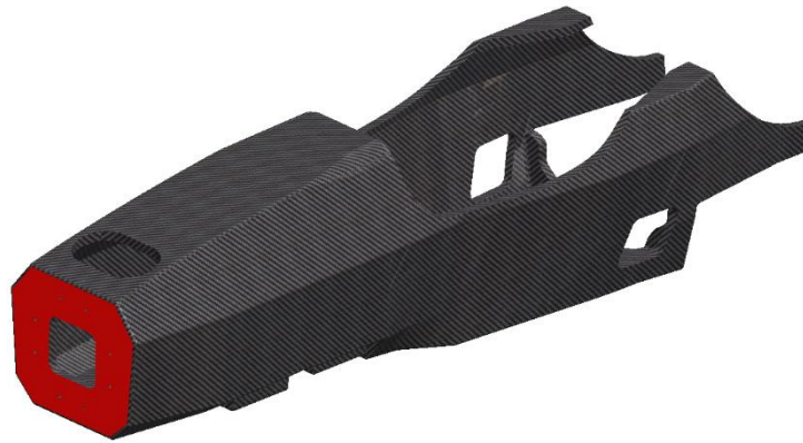
Figure 46 - Front bulkhead region highlighted
