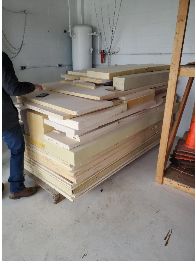
Figure 144 - Stack of tooling board at Battle Creek airport
