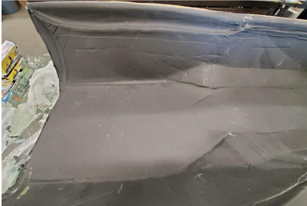
Figure 175 - Failed final cure of BR20 lower mold
