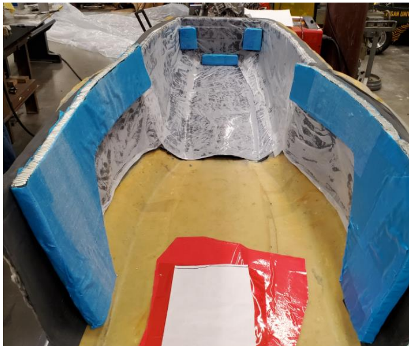
Figure 167 - Properly wrapped aluminum core
