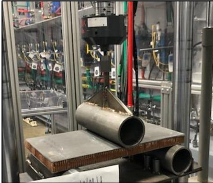
Figure 118 - Three-point bend test conducted on MTS
