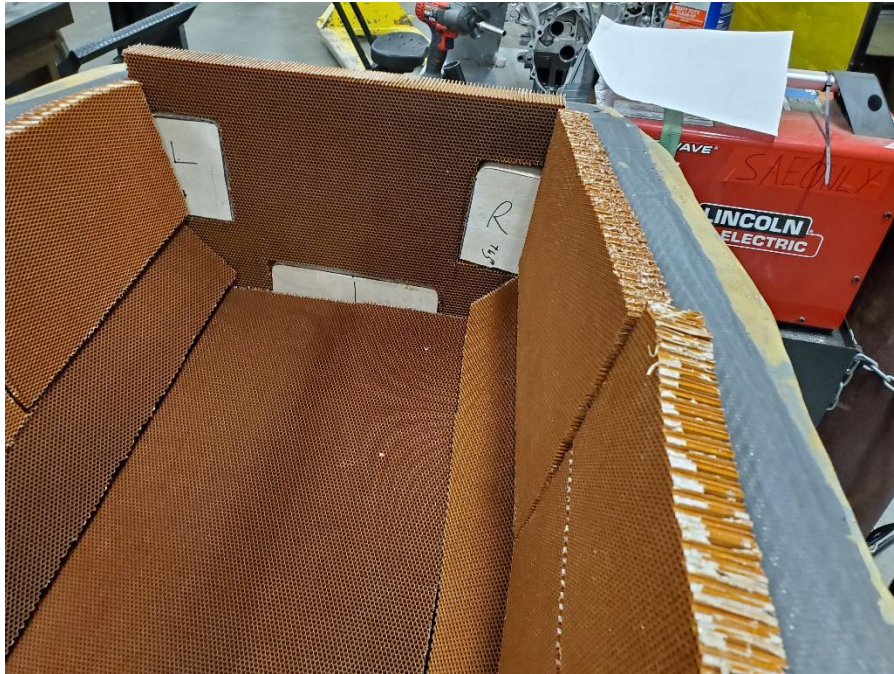
Figure 165 - BR20 Nomex and balsa core placement
