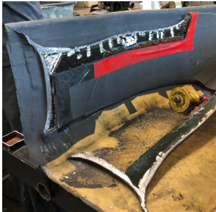
Figure 176 - BR20 with affected laminate removed
