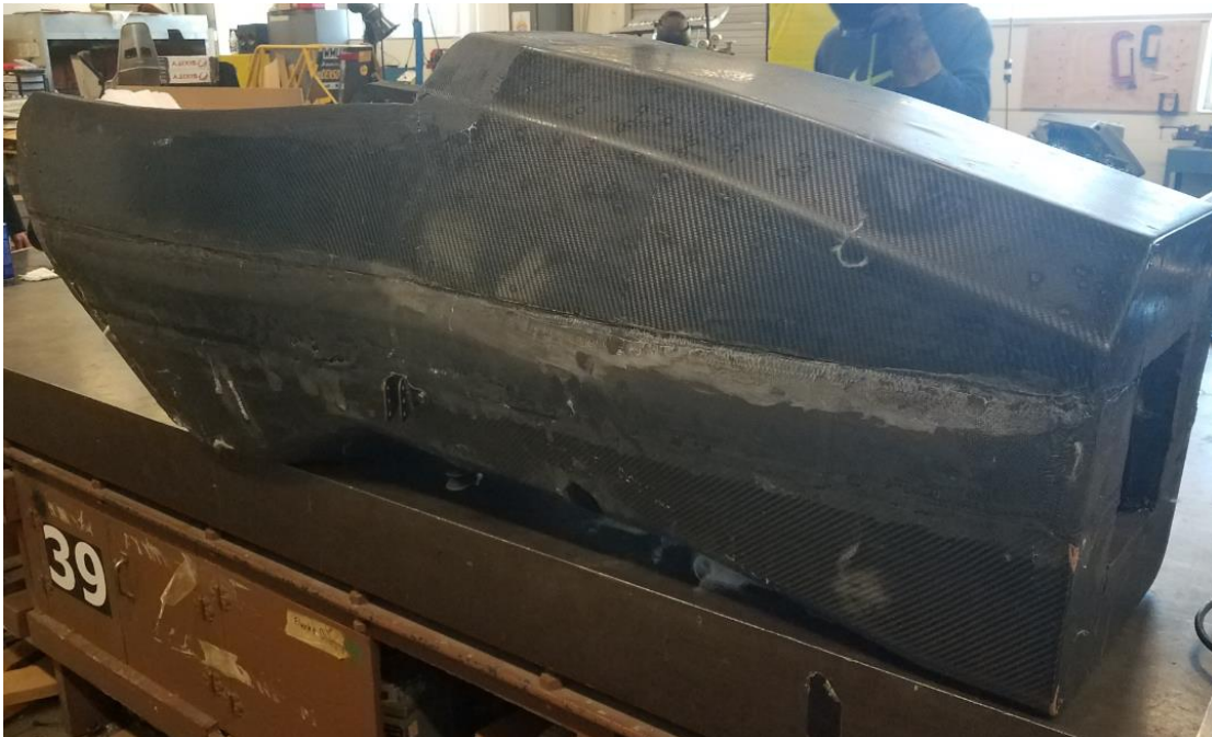
Figure 190 - BR20 with front hoop lap joint and core coverage
