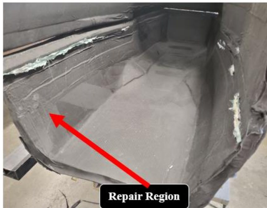
Figure 181 - BR20 cured repair
