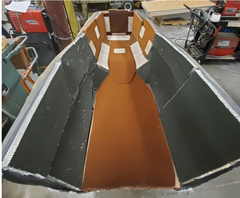
Figure 166 - BR20 dry fit of core materials
