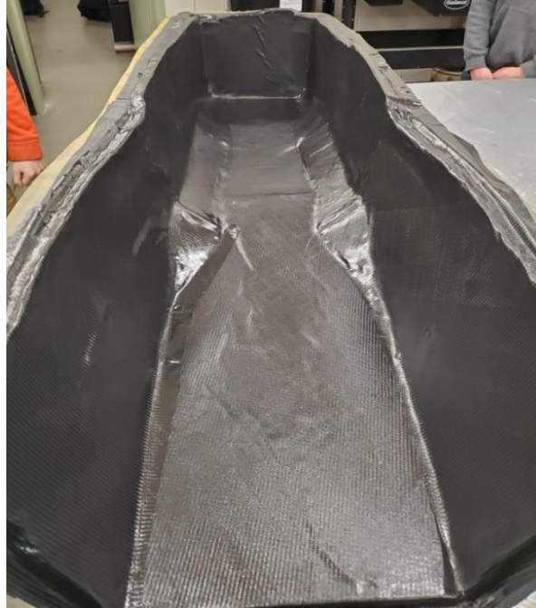
Figure 171 - BR20 lower mold with all laminate placed
