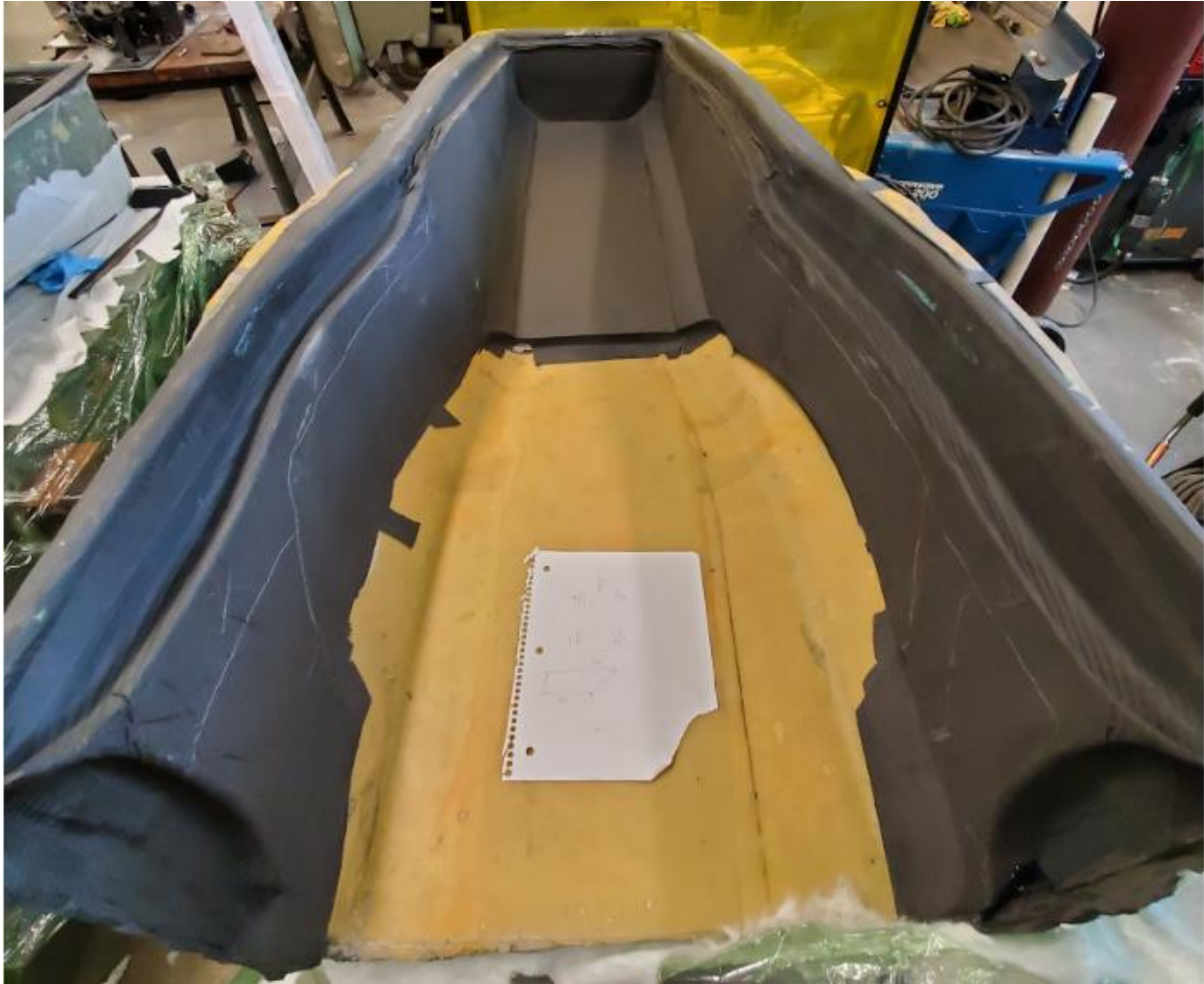
Figure 172 - BR20 deformed upper core
