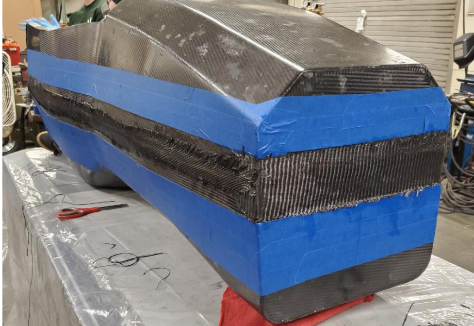
Figure 185 - BR20 uncured lap joint
