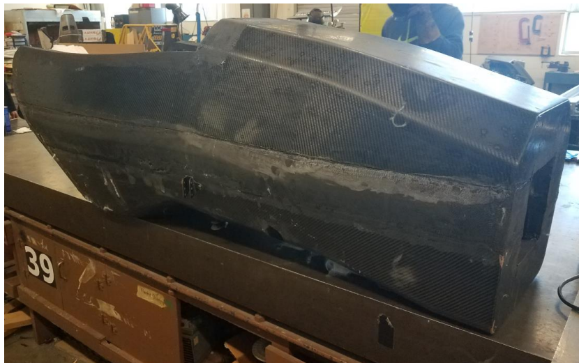
Figure 13 - BR19 low quality lap joint
