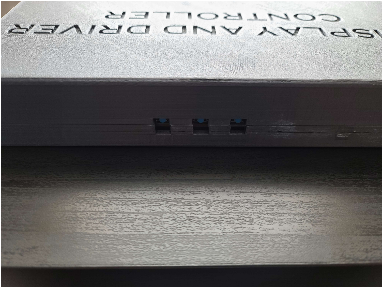
Figure F3: PCB Enclosure Front View of Switches
