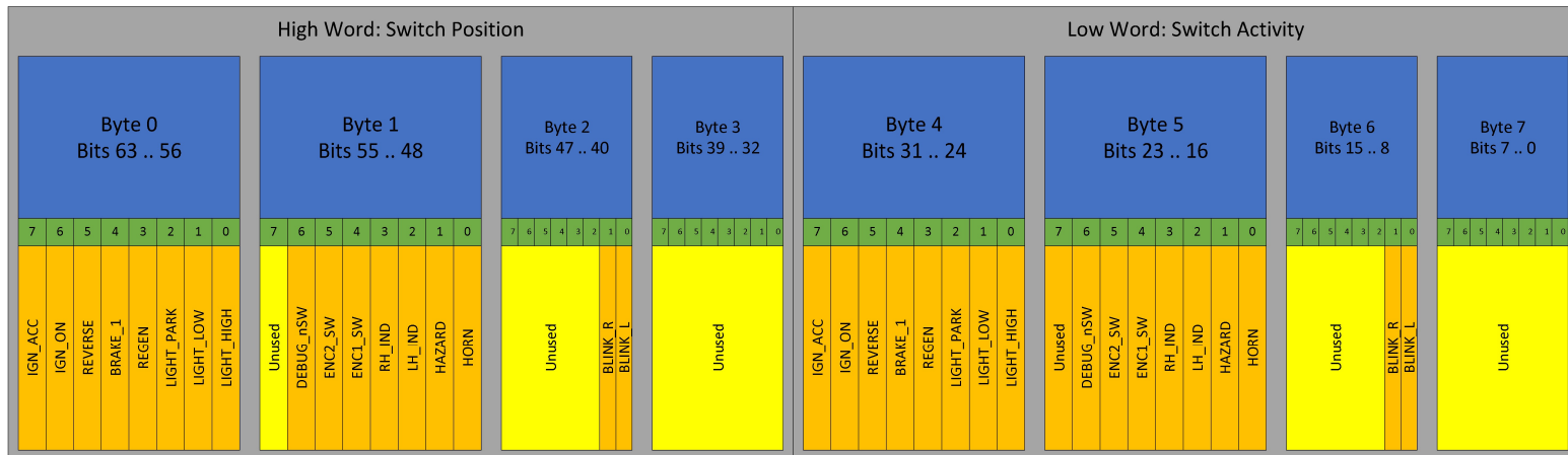
Figure E4: DC_SWITCH Command The above layout shows what the actual message looks like on the CAN bus
