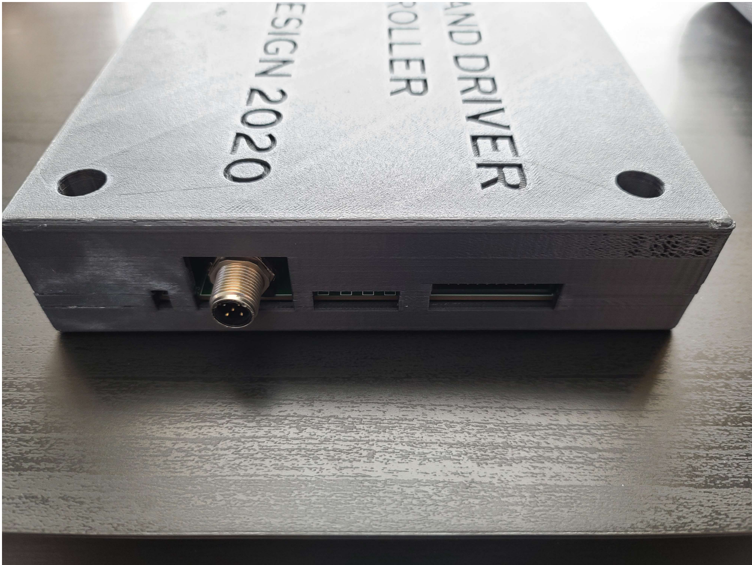
Figure F2: PCB Enclosure Left View of Connectors
