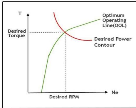
Figure 5: Desired torque and desired RPM lookup
