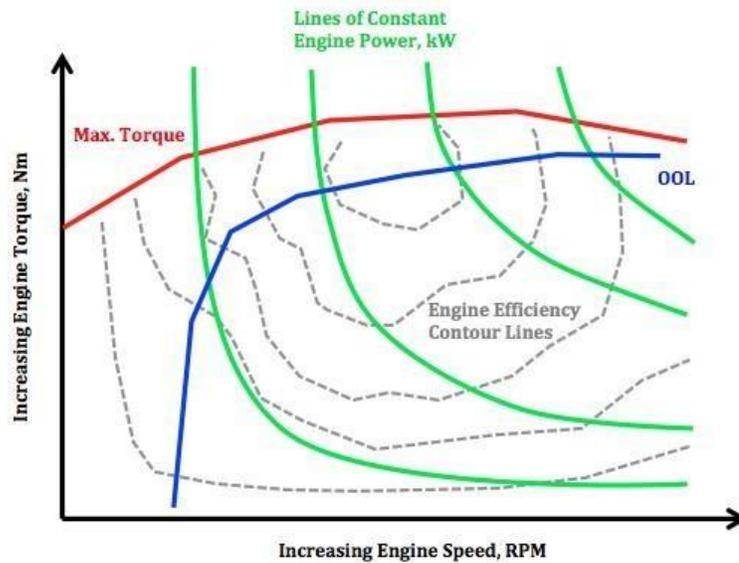
Figure 1: Sample speed vs. torque map with the derivation of an engine OOL
