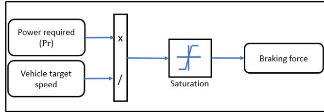
Figure 6: Braking force calculation
