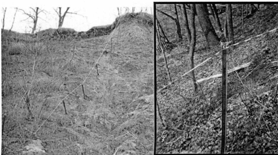
Figure 1. One of the pole-and-cable displacement monitoring lines installed on a Lake Michigan slump system. Each line is surveyed individually by measuring the distance between poles, cable height above ground at each pole, cable sag angles between poles, and pole inclination angles in both the strike and dip direction of the slope.
