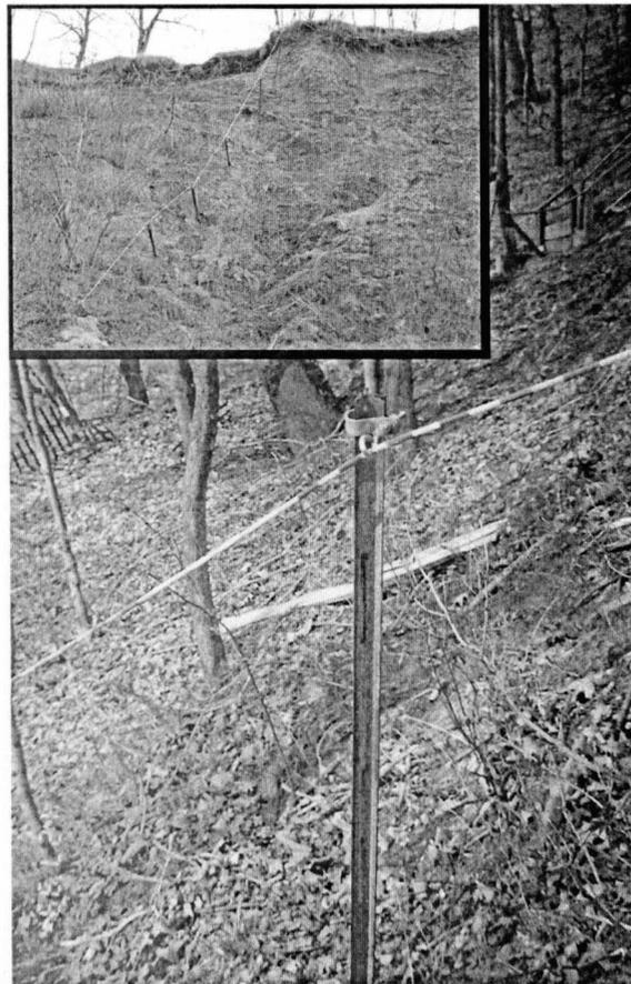
Figure 10. The pole-and-cable slope displacement monitoring system (described in Chase et al., 2001a). Measurements from the system are used to compute neural
