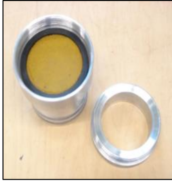
Figure 5. Specimen in Gasket within Holder Accessory
