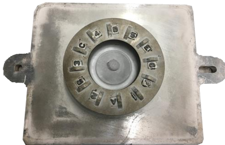
Figure 67. Matchplate Pattern for the Surface Defect Casting Trial.
