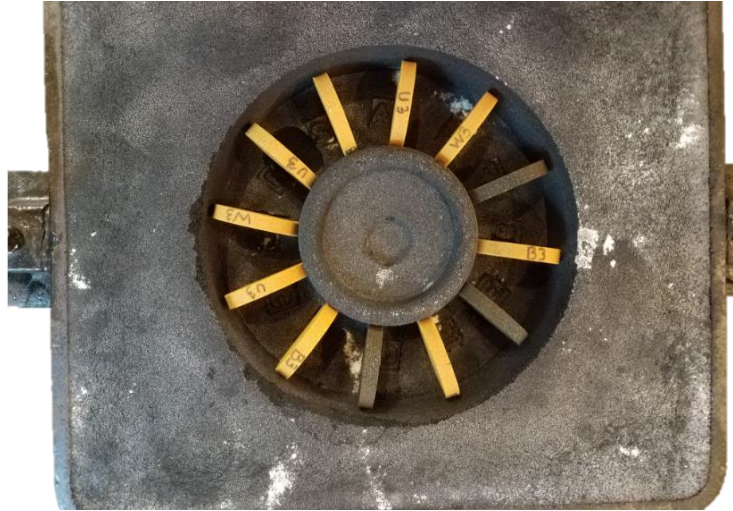
Figure 68. The Disc-shaped Specimens Placed on the Core Prints in the Drag Half of the Mold
