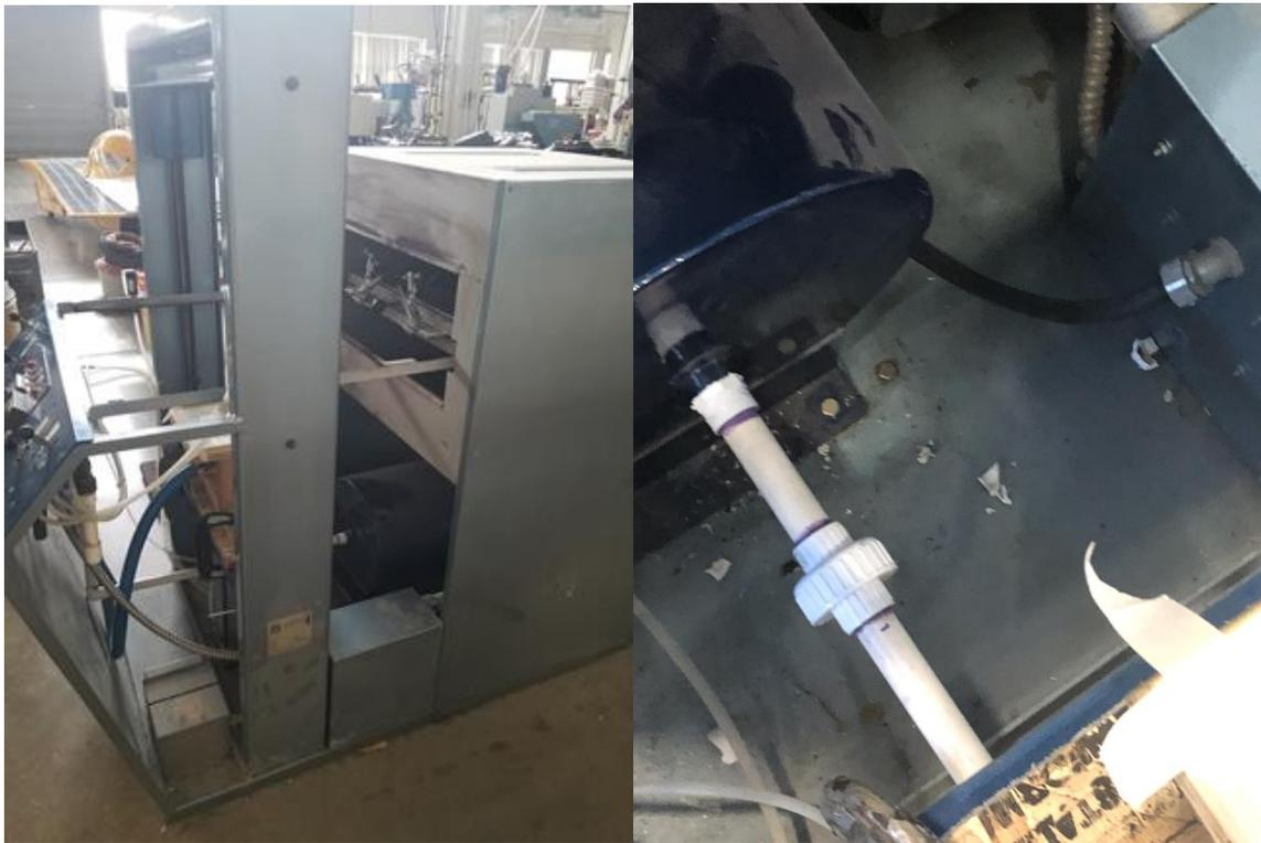
*Figure 6: Vacuum Pump System Within the Thermoforming System (Left) and By Itself (Right)*
