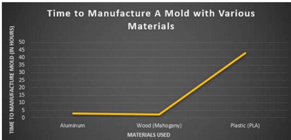
*Figure 12: Times to Manufacture a Mold with Various Materials*
