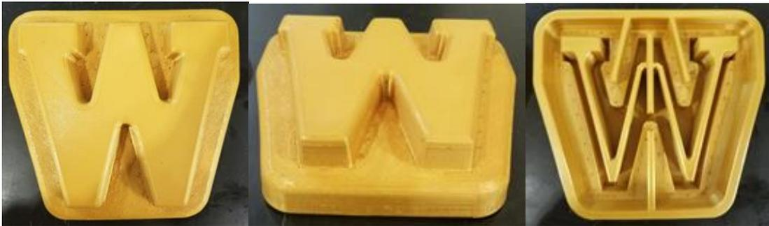
*Figure 8: Final Mold Design Remodel with Adequate Supports (the "Support Skeleton")*
