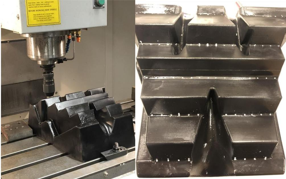
*Figure 1: Prototype Mold Mounted in CNC*
