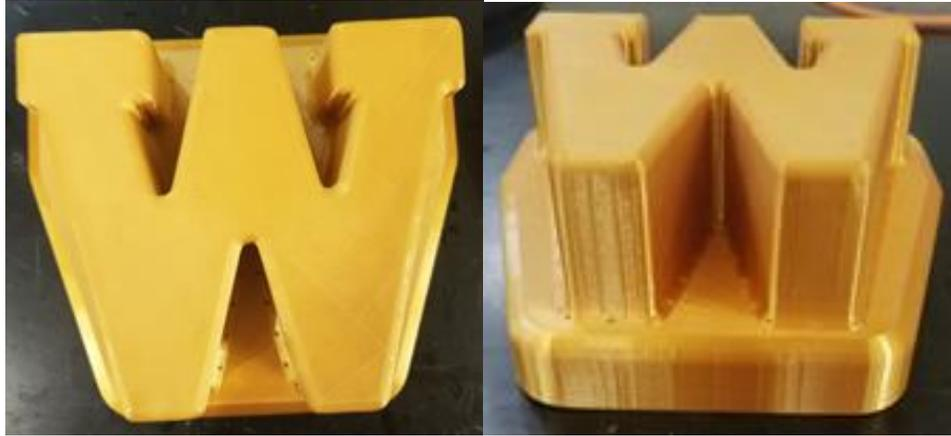
*Figure 5: First Complete Mold Redesign – Too Large*
