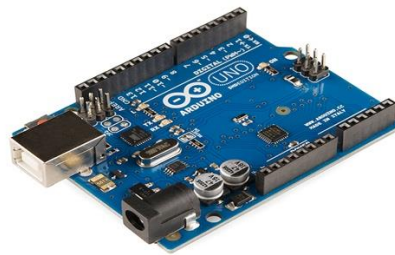
Figure 7: Arduino UNO Microcontroller Board
