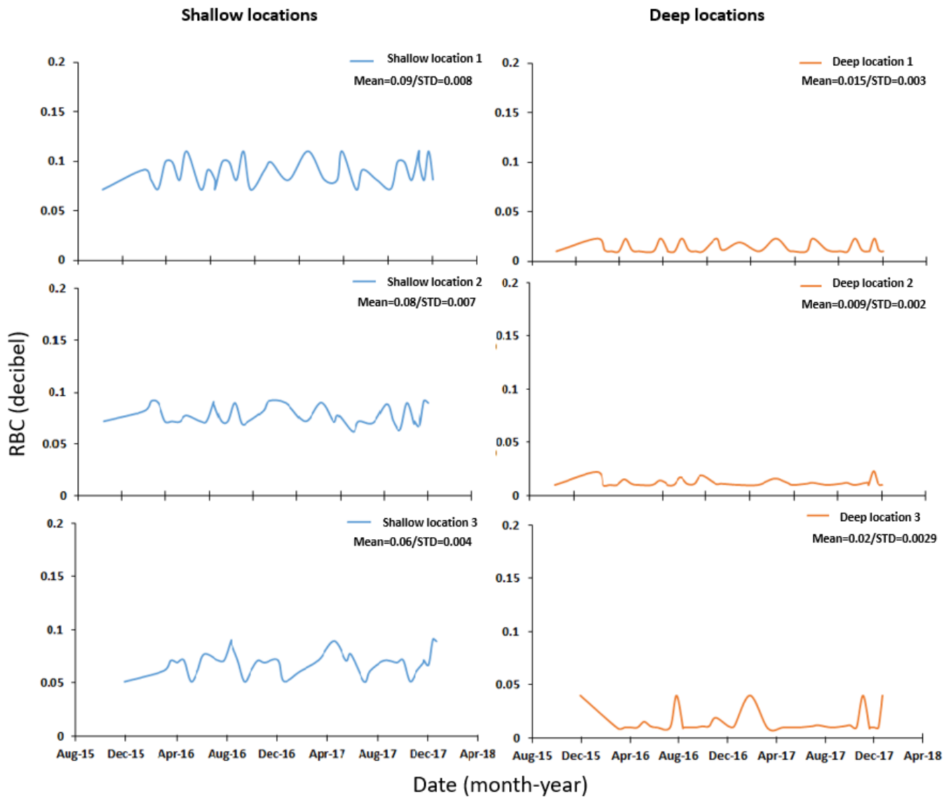
Figure 10. Time series of RBC. In decibel derived from Sentinel-1 over three areas characterized by shallow groundwater and three other locations characterized by deep groundwater.
