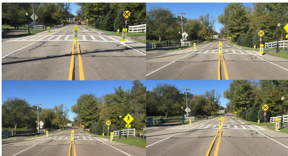
Figure 6. Gateway widths at Garden Avenue 12 ft (top left), 14 ft (top right), 16 ft (bottom left), and 18 ft (bottom right).
