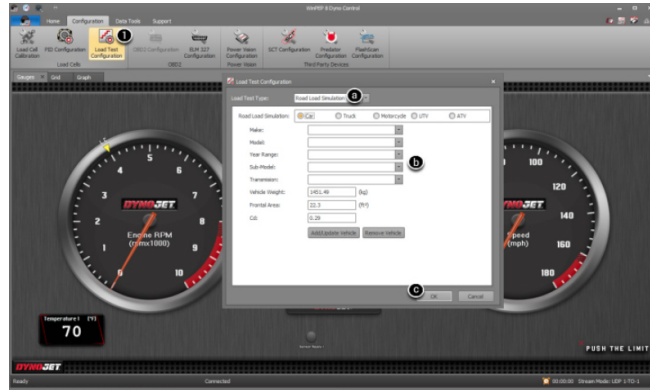
Figure 9.10: Road load control module configuration from chassis dynamometer manufacturer (dynojet-224xLC).
