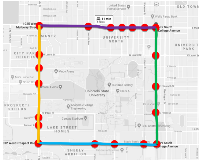
Figure 5.3: Selected data drive-cycle; drive order was purple, yellow, blue, then green, red circles represent traffic signals
