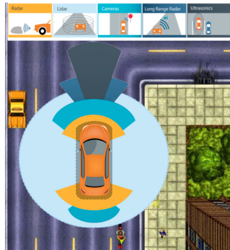
Figure 9.4: An illustration of the type and placement of sensors in an autonomous vehicle that enable the vehicle to perceive its surroundings.
