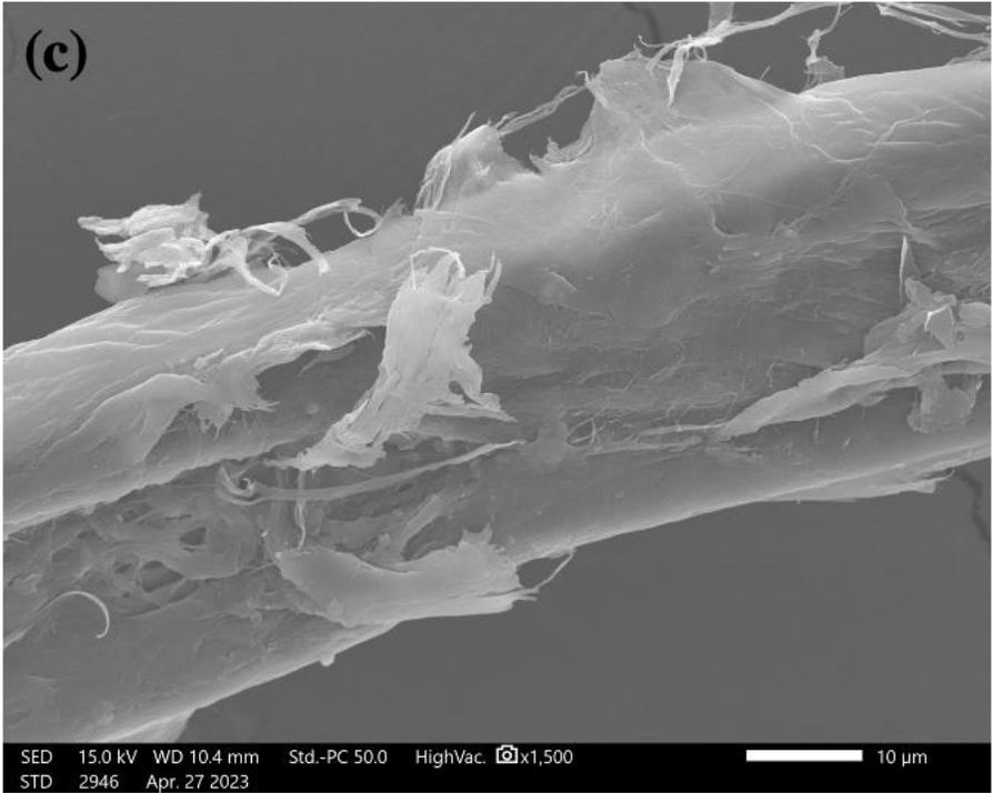
Figure 5.7. SEM images of untreated secondary fibers refined at 6000 revolutions, (a) paper surface network, scale bar is 100 microns, (b) fiber-fiber contact, scale bar is 20 microns, and (c) fiber surface, scale bar is 10 microns.
