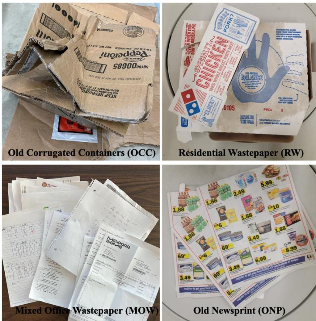
Figure 5.1. Recycled OCC and ONP collected from local paper recycling mill, residential wastepaper RW collected from curb side, and MOW collected from office.
