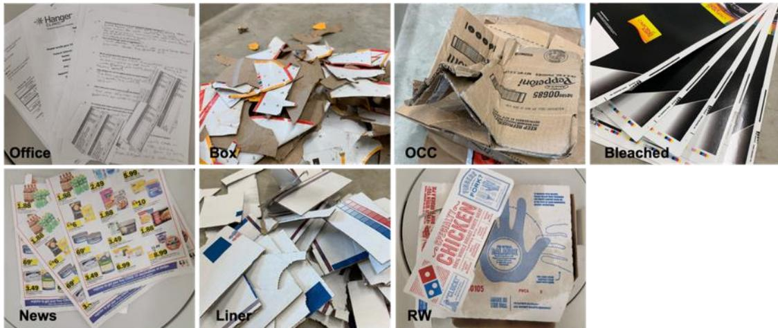
Figure 3.1. Recycled paper raw materials collected from local paper mill and curb-side stream.
