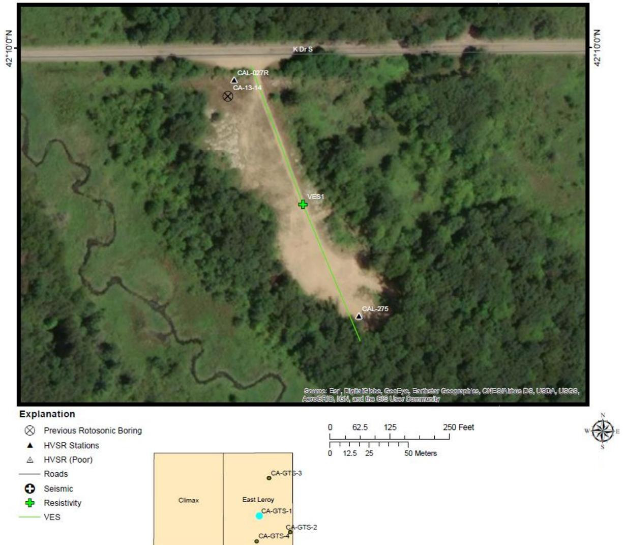
**Figure 31.** Map of CA-GTS-1 displaying resistivity sounding locations in a sand and gravel pit near K Drive S. Note the location of several HVSr stations and boring CA-13-14.
