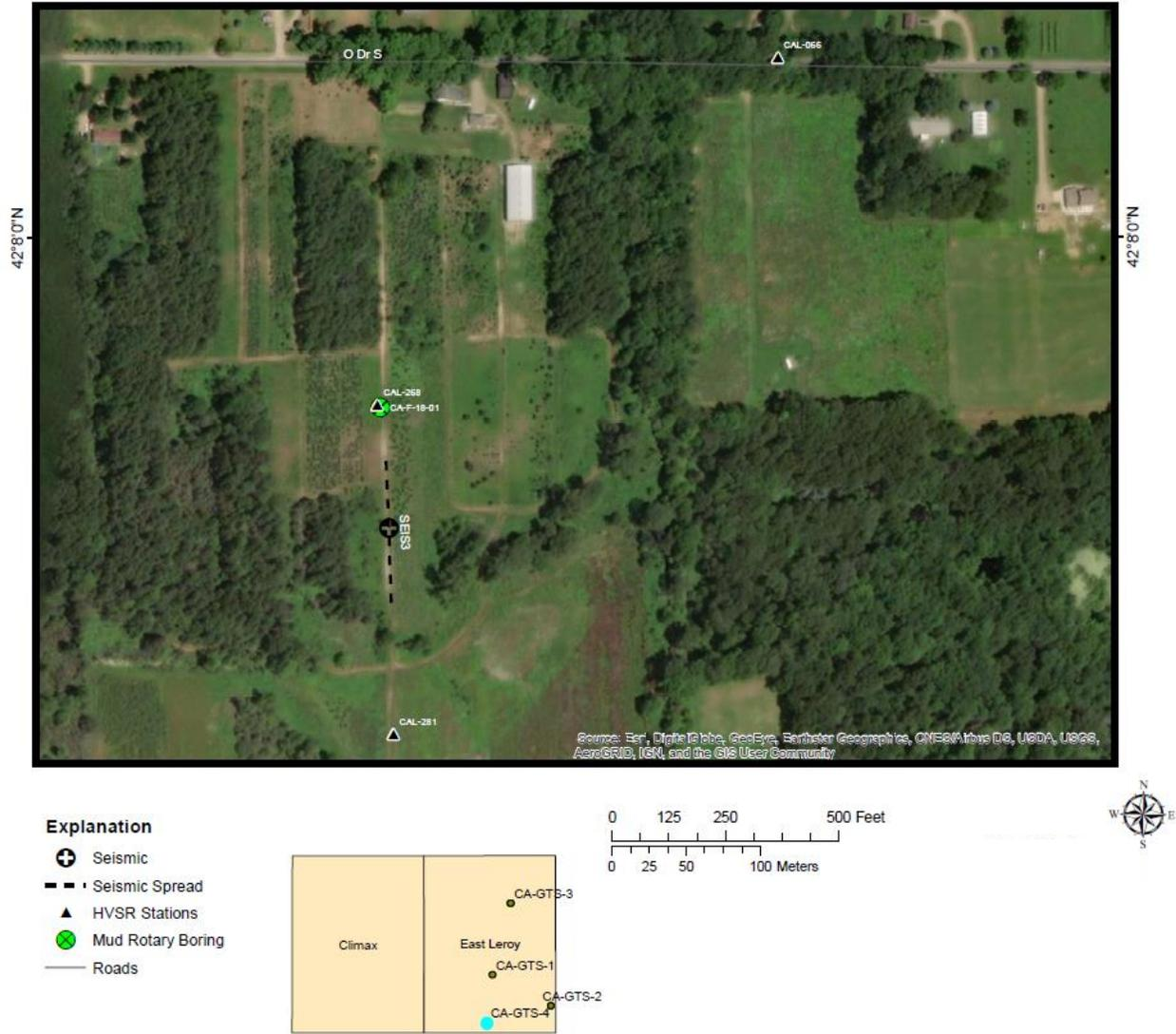
**Figure 42.** Map of CA-GTS-4 displaying seismic survey line along a dirt road near O Drive S. Note the location several HVSR stations and boring CA-F-18-01.
