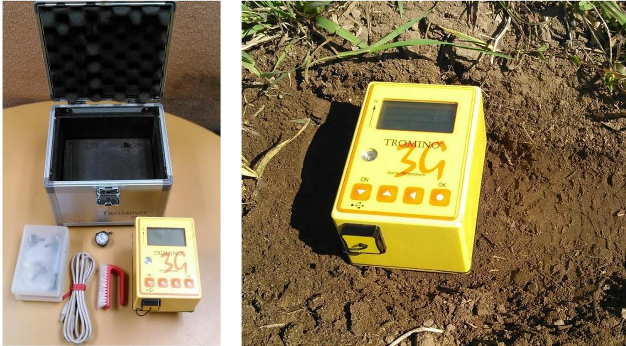
**Figure 6. Left:** Tromino equipment case. Materials include: spare AA batteries, alternative hard surface spikes, USB connection cable to download field data to a computer, compass to orient the instrument north, brush to clean coupling spikes of debris, and the Tromino Zero 3G instrument (Serial no. TZ3-0032/01-15). **Right:** The “planted” Tromino unit prepared to make a station recording.
