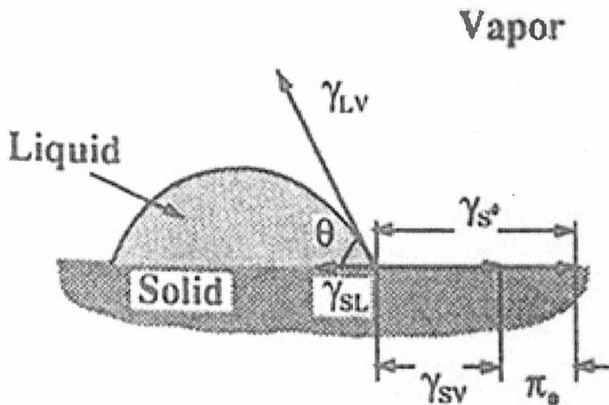
Figure 1. Components of Interfacial Tension and Contact Angle
