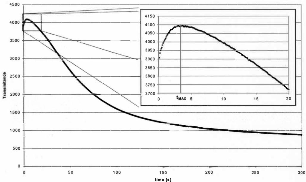
Figure 13. Ultrasound Transmittance Versus Time of Liquid Penetration
