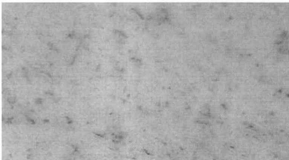
Figure 7. Stain Test on a Release Paper.
