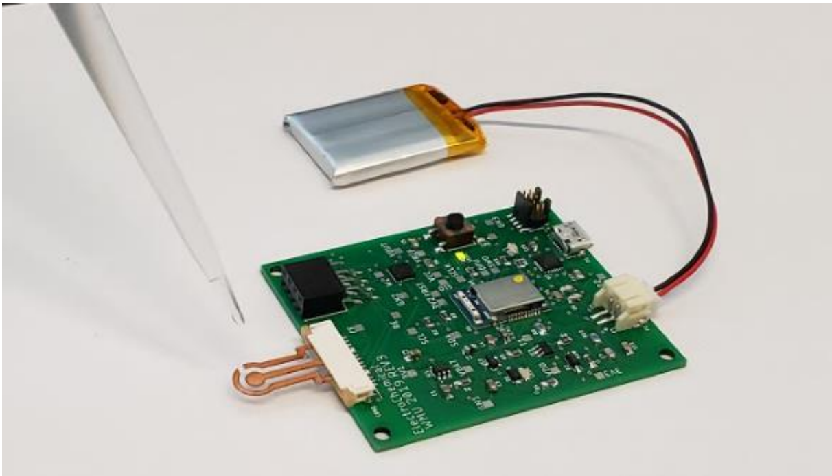
Figure 3.17 Pipette to drop the glucose sample onto the sensor.
