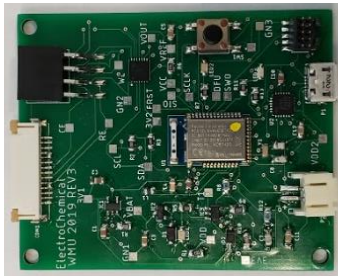
Figure 3.15 Photograph of the Portable Electrochemical System.
