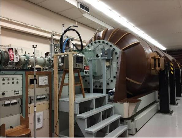
Figure 7. 6.0 MV Tandem Van de Graaff Accelerator at WMU
