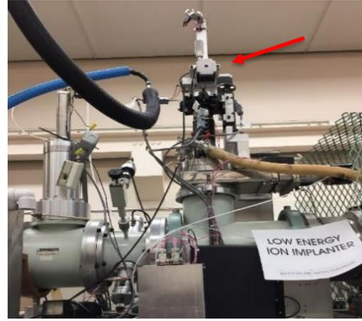
Figure 8. The XY stepper motors
