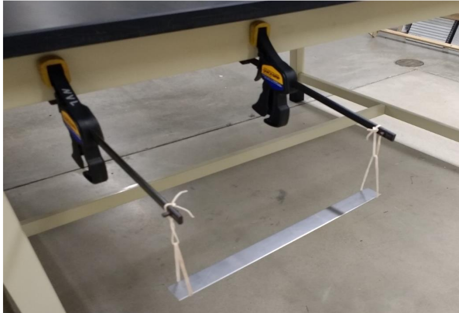
Figure 7.8 Creation of free-free boundary conditions for a flat beam
