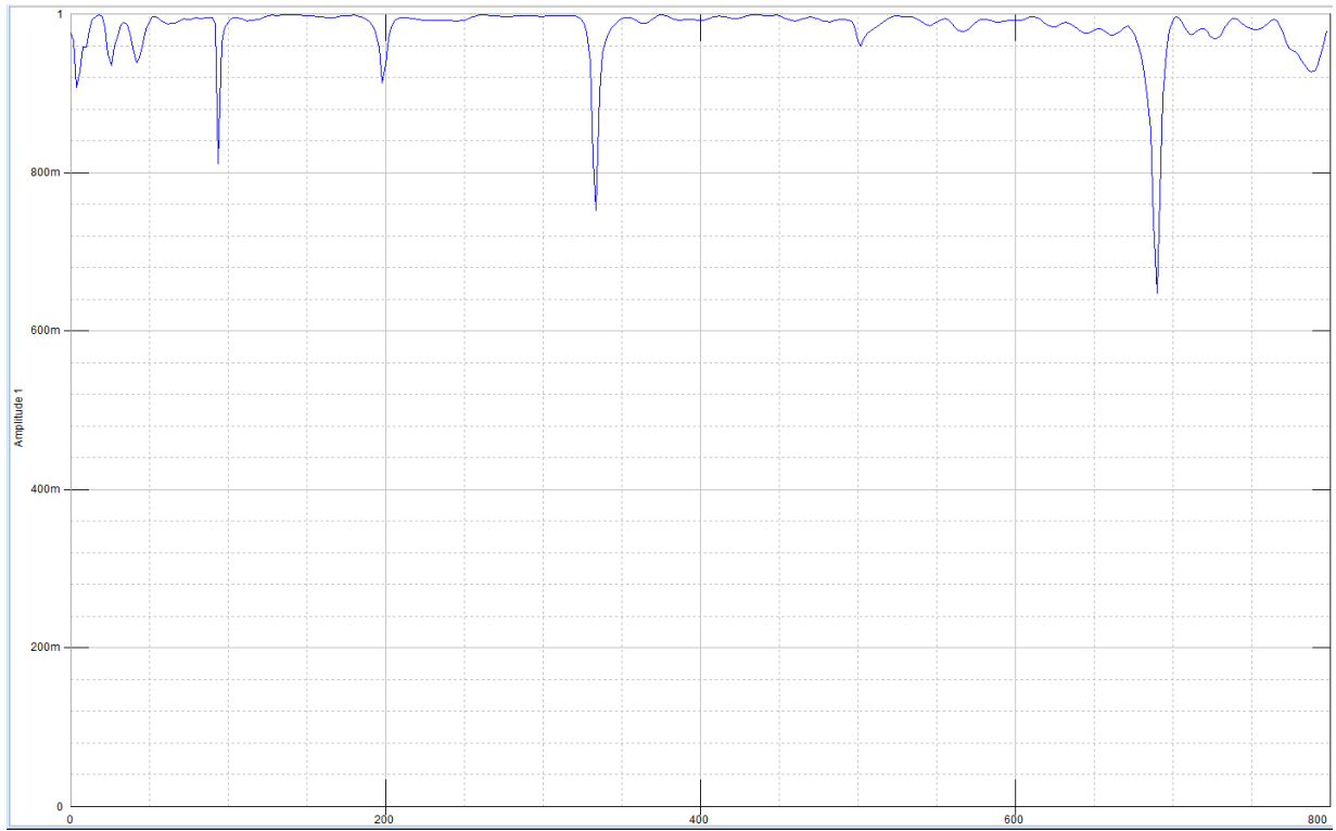
Figure 7.12 Example of good coherence with the dips signifying resonances
