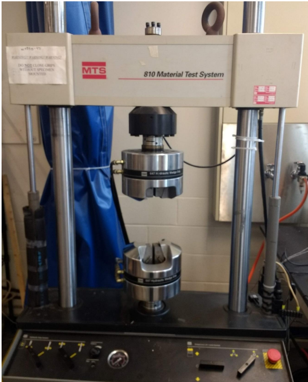
Figure 3.5 The MTS 810 Material Test System used to perform the uniaxial tension test
