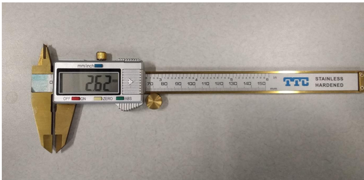
Figure 5.4 Digital caliper (Range 0-150 mm and least count 0.01 mm)
