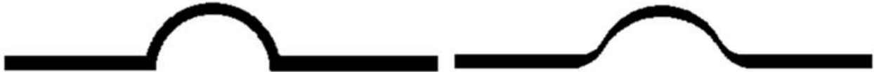
Figure 1.5 Comparison of dimple with uniform thickness (left) and dimple with non-uniform thickness (right)
