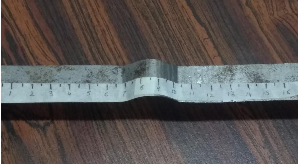
Figure 5.9 Paper tape on the beam acting as a measuring scale and centerline marker
