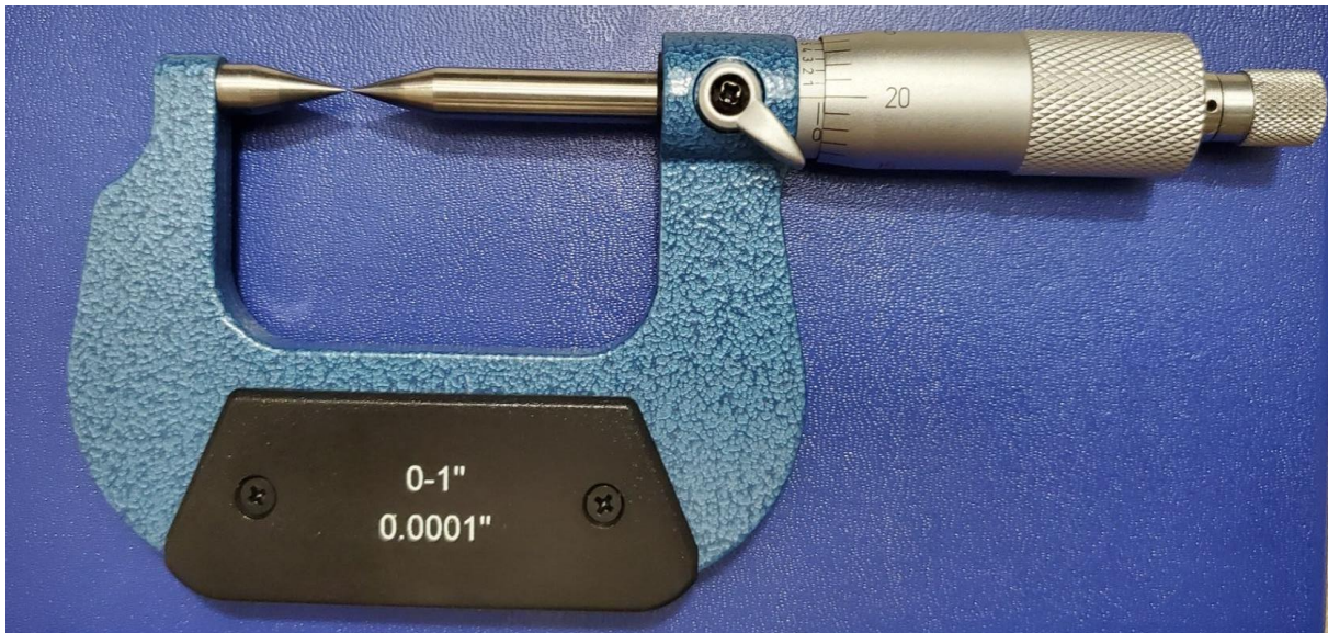
Figure 5.1 Point micrometer (Range: 0-1" and least count 0.0001")
