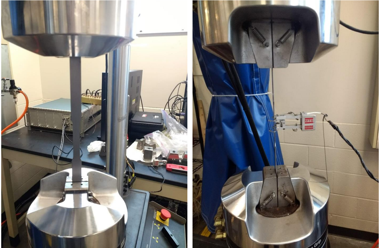
Figure 3.6 Front view (left) and side view (right) of test specimen clamped in the jaws of the machine with the attached extensometer visible as well
