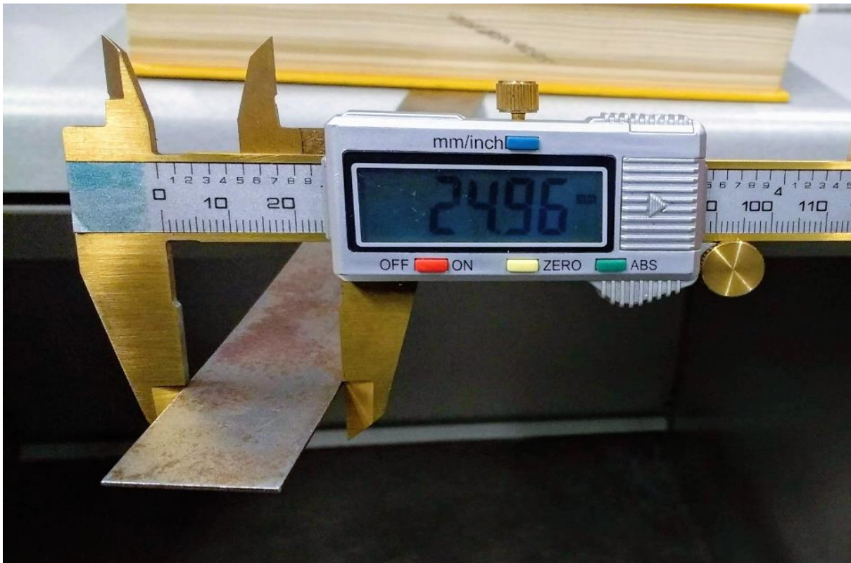
Figure 5.6 Measurement of beam width using a digital caliper
