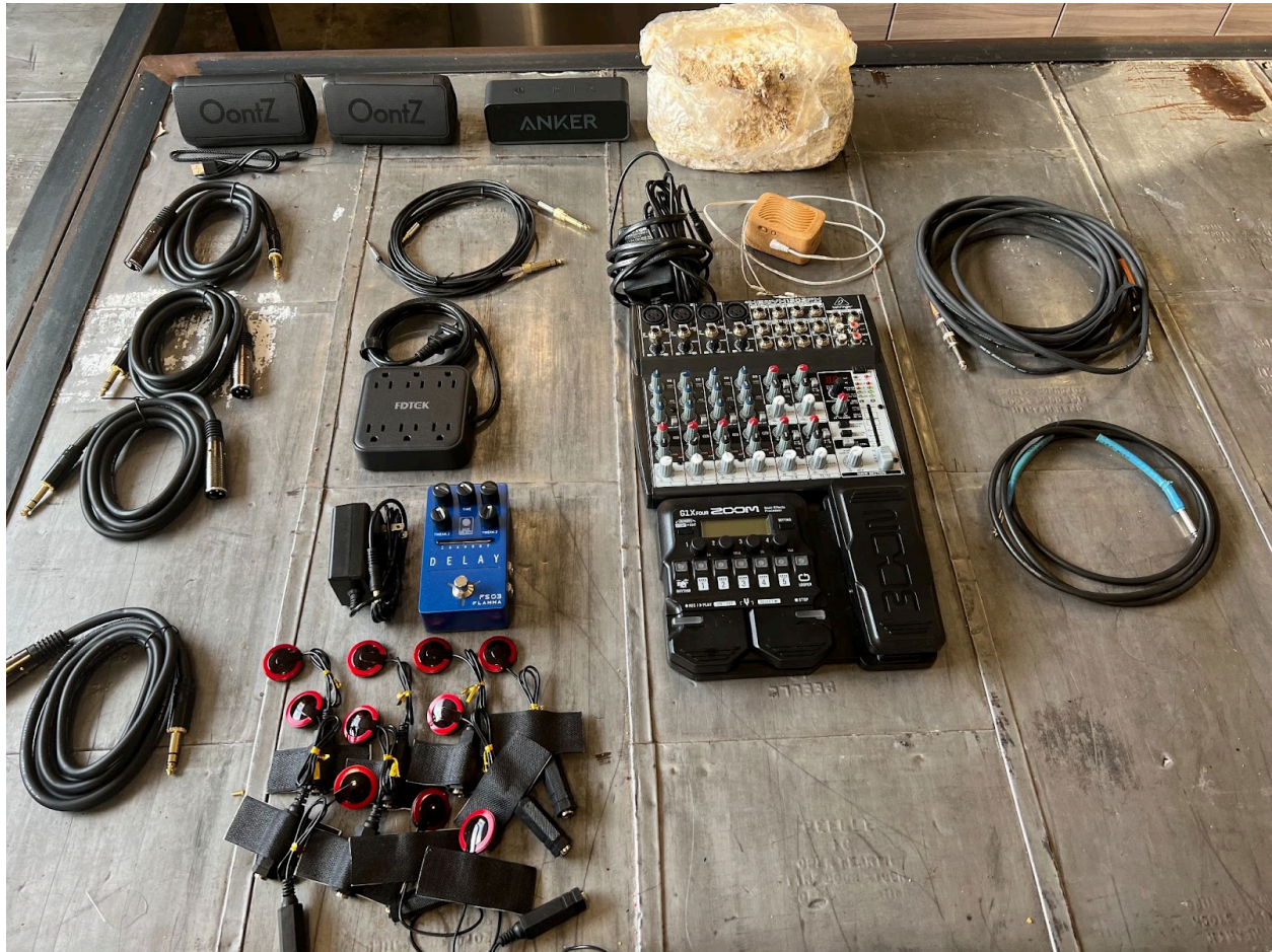
Figure 31. Tech used (left to right, top to bottom): Two OontZ Bluetooth speakers, one Anker speaker, a fruiting block of fungi for demonstration, four TRS-XLR cables, two aux cables with TRS adapters on one end each, a power strip, a delay pedal with power adapter, 10 contact microphones, a PlantWave, a Behringer 4-channel mixer with power adapter, a Zoom multi-effects pedal, and several TRS-TRS cables. Not pictured: portable battery jumper, Galaxy Audio JIB/S 4-way splitter. In addition, I added a set of powered studio speakers in lieu of using only Bluetooth speakers.
