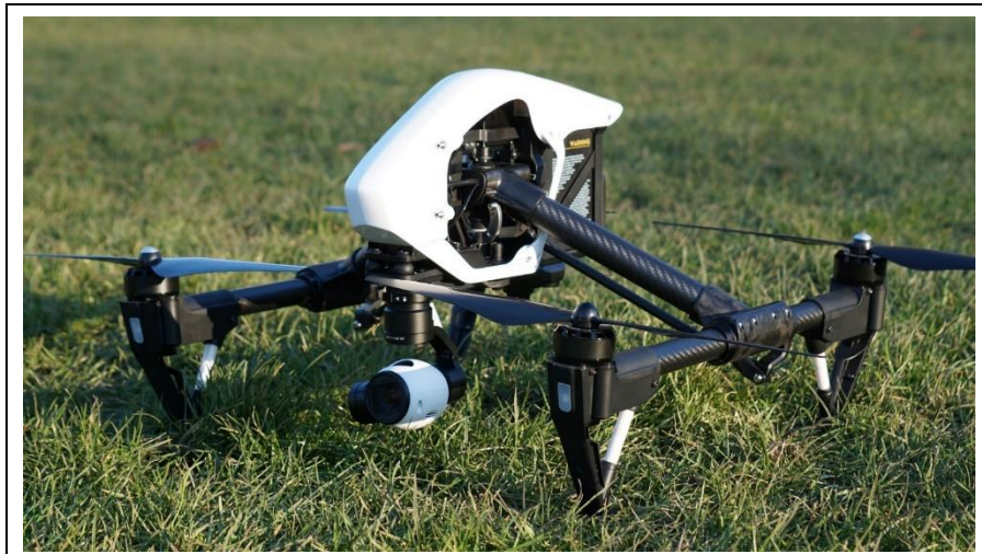
Figure 5. DJI Inspire 1 UAS with camera and gimbal system used to photograph Hagar Park/Beach (Simon, 2015).
