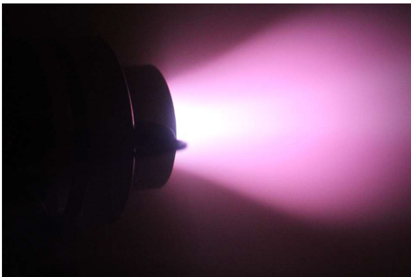
Figure 28: Operation of the WECR thruster during characterization at 1 SCCM and 20 W.
