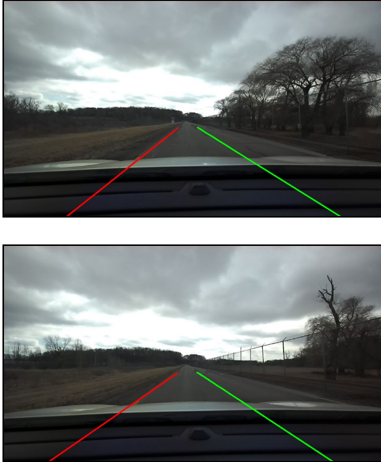
Figure 24. Two examples of Eaton Proving Grounds camera frames from straight road segments with high-definition map lane line data overlaid on artificially occluded lane lines. These show well-aligned lane lines.
