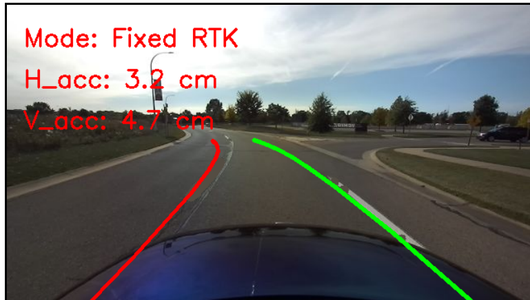
Figure 27. Campus Drive camera frame from a curved road segment with high-definition map lane line data overlaid on artificially occluded lane lines. Deviation from true lane lines occurs in this curved road segment due to the insufficient sampling rate of the GNSS heading sensor.
