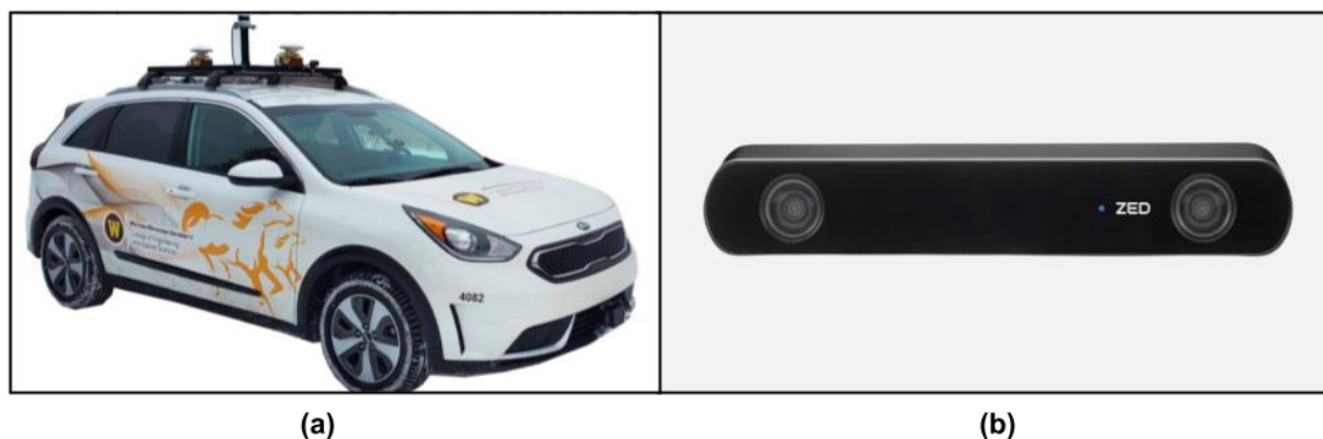
Figure 8. (a) Kia Niro Instrumented Research Vehicle, (b) ZED 2 stereo camera.
