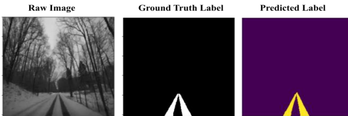
Figure 5. CNN output (The raw image is on the left, the labeled segmentation mask is in the middle, and the predicted segmentation mask from the CNN is on the right)
