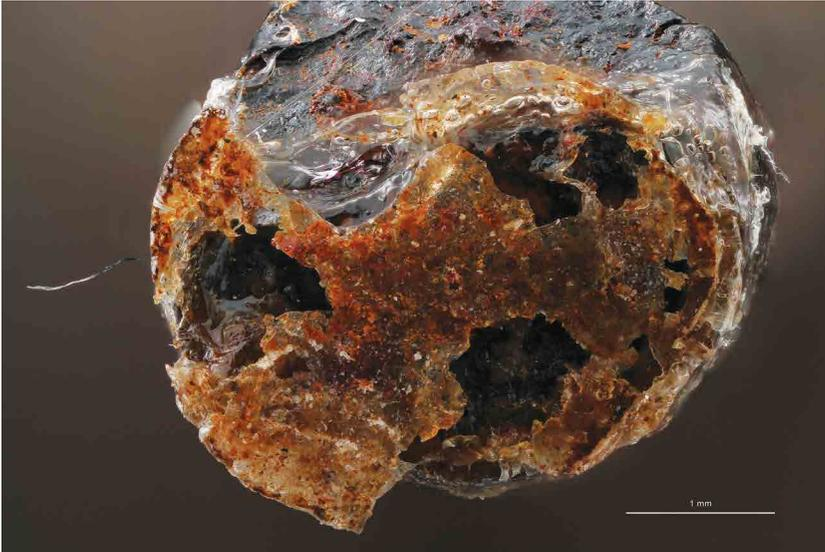
**Figure 15.2.** Edge of an ancient copper nail. The nail was broken and restored, but broke again after some time. The glue used to fix the nail is clearly visible.
