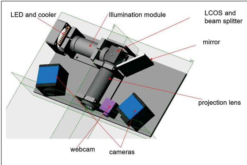
**Figure 22.1. Schematic of a typical compact structured light scanner with two cameras (webcam only for alignment) developed by the Centre for Sensor, Instruments and System Development at the Universitat Politècnica de Catalunya (UPC-CD6). © UPC-CD6, 2010.**
