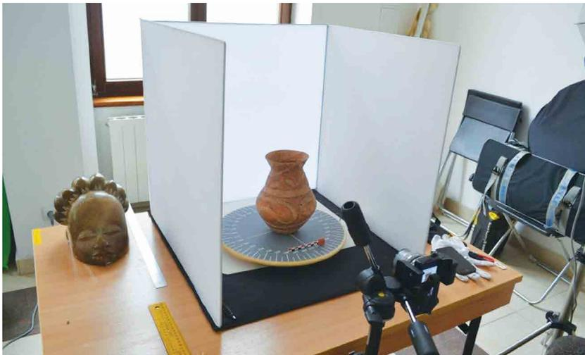
**Figure 6.2.** Setup for photogrammetric acquisition of the ceramic vases.
