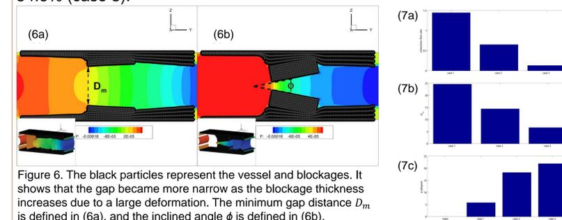
Figure 6. The black particles represent the vessel and blockages. It shows that the gap became more narrow as the blockage thickness increases due to a large deformation. The minimum gap distance  $D_m$  is defined in (6a), and the inclined angle  $\phi$  is defined in (6b).
