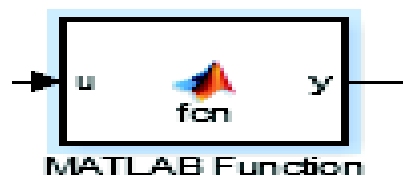
Figure 4.2 Matlab® user defined function block
