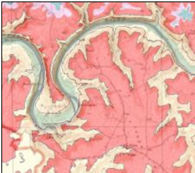
Figure 3: Topographic map with geology overlays displaying areas of sandstone cap (red and pink) and areas of exposed limestone (yellow).
